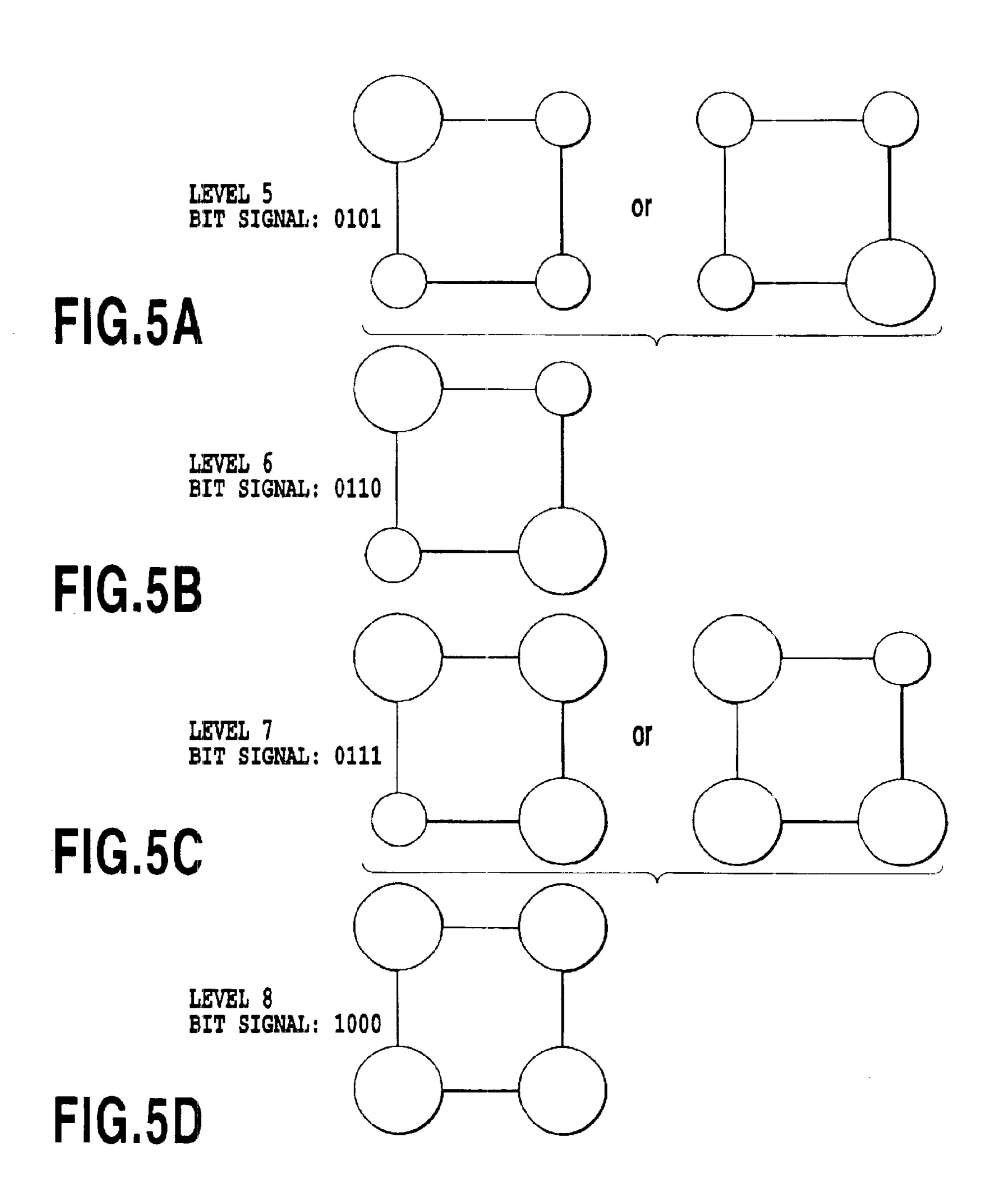
RELATIONSHIP BETWEEN INPUT LEVEL AND LANDED RATE OF INK IN THE CASE WHERE SAME PLANE DATA FOR RESPECTIVE LARGE AND SMALL DROPLETS SAME INDEX PATTERNS FOR RESPECTIVE LARGE AND SMALL DROPLETS) ARE USED
