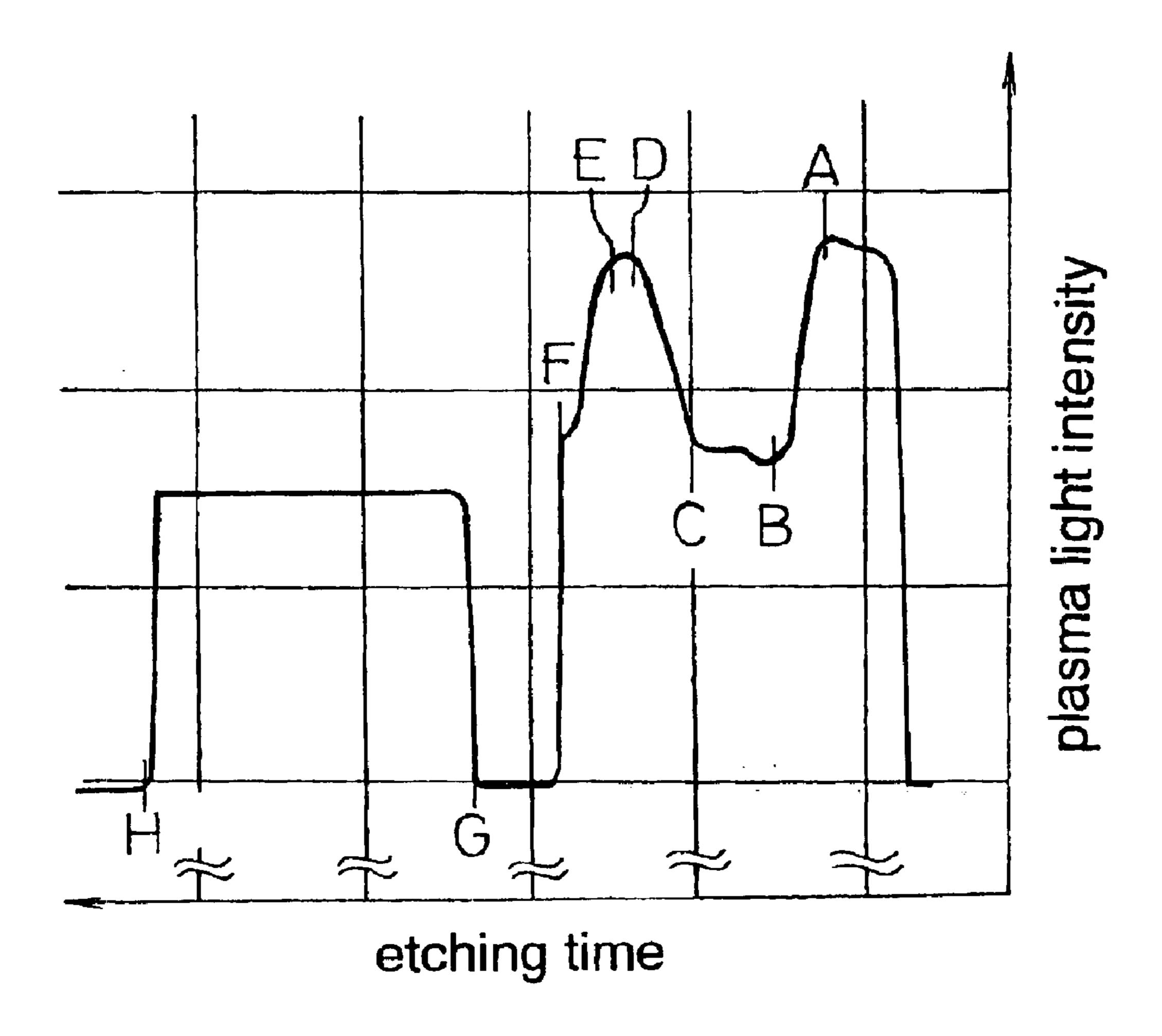
~A: Titanium etching A~B: Titanium/Aluminum etching
