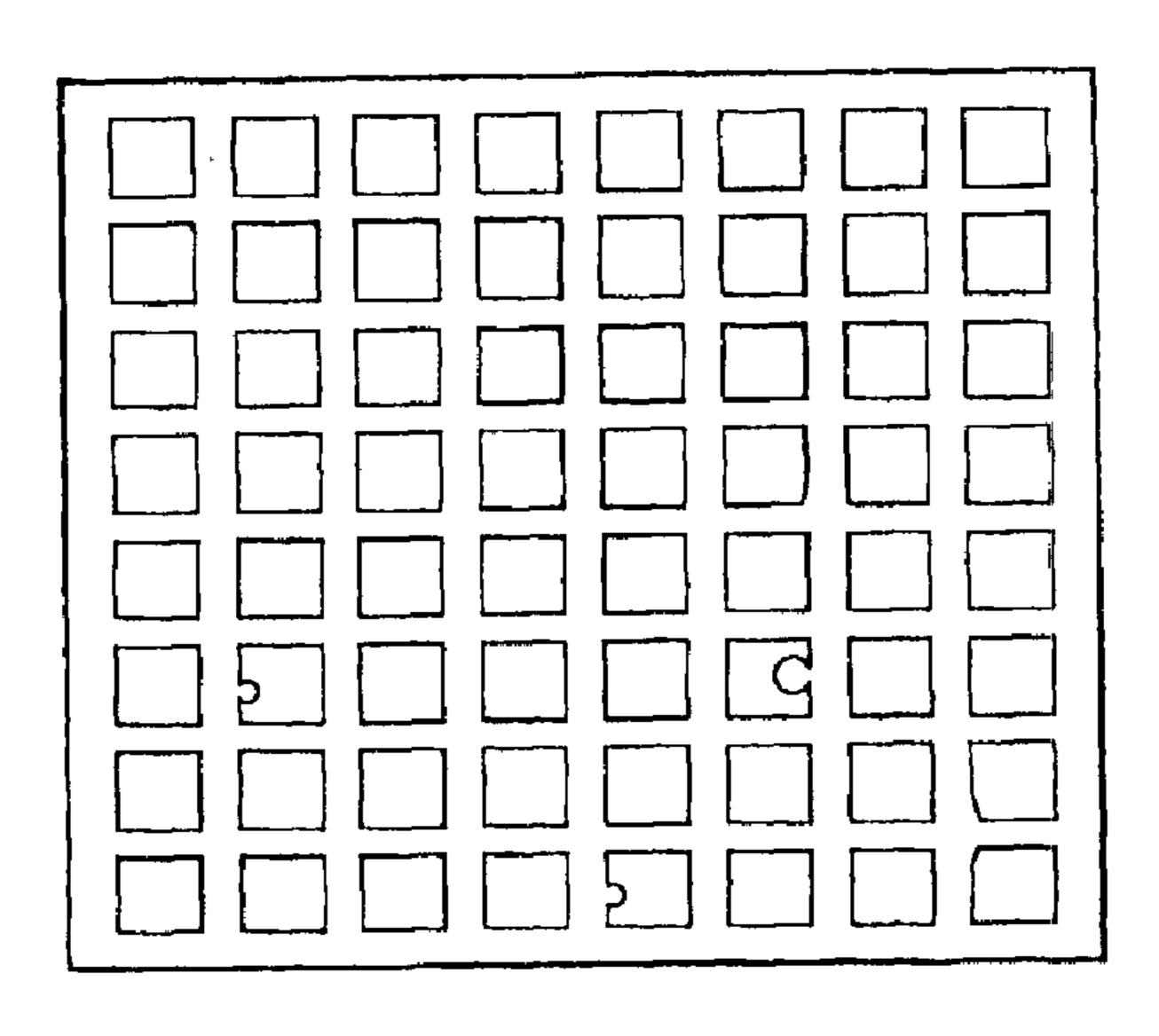
FIG. 7 POLYMER LIGHT EMITTING DISPLAY WITH PROTECTIVE LAYER AFTER 288 HOURS OF EXPOSURE TO 50°C AND 95% RELATIVE HUMIDITY
