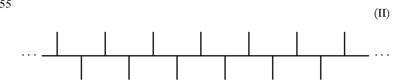
A polymer chain showing no regular order of repeating unit configurations is an atactic polymer. In commercial applications, a certain percentage of atactic polymer is typically produced with the isotactic form. It is highly desirable to control the atactic form at a relatively low level.
