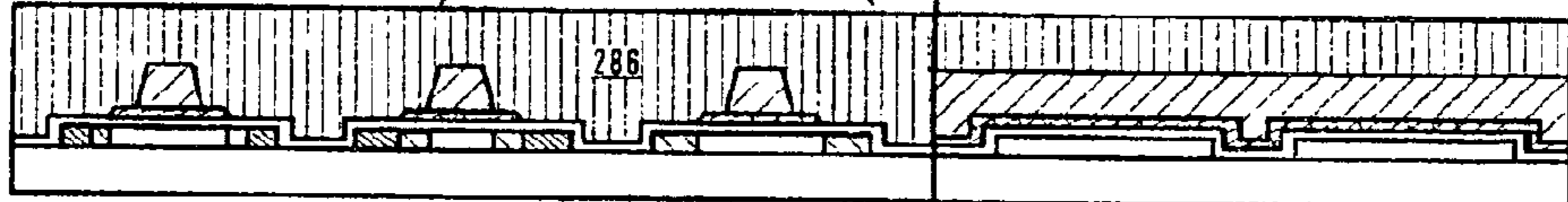
Fig.3F GATE METAL ETCHING 3 / DOPING 3
