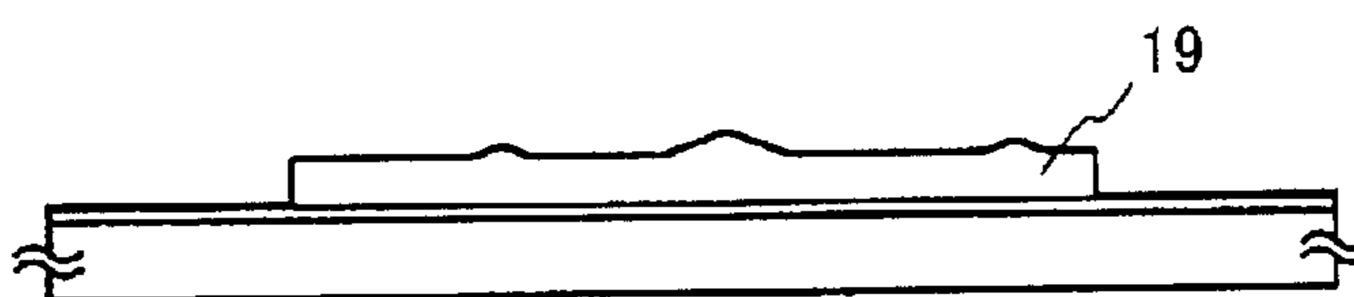
Fig. 3E formation of semiconductor film
