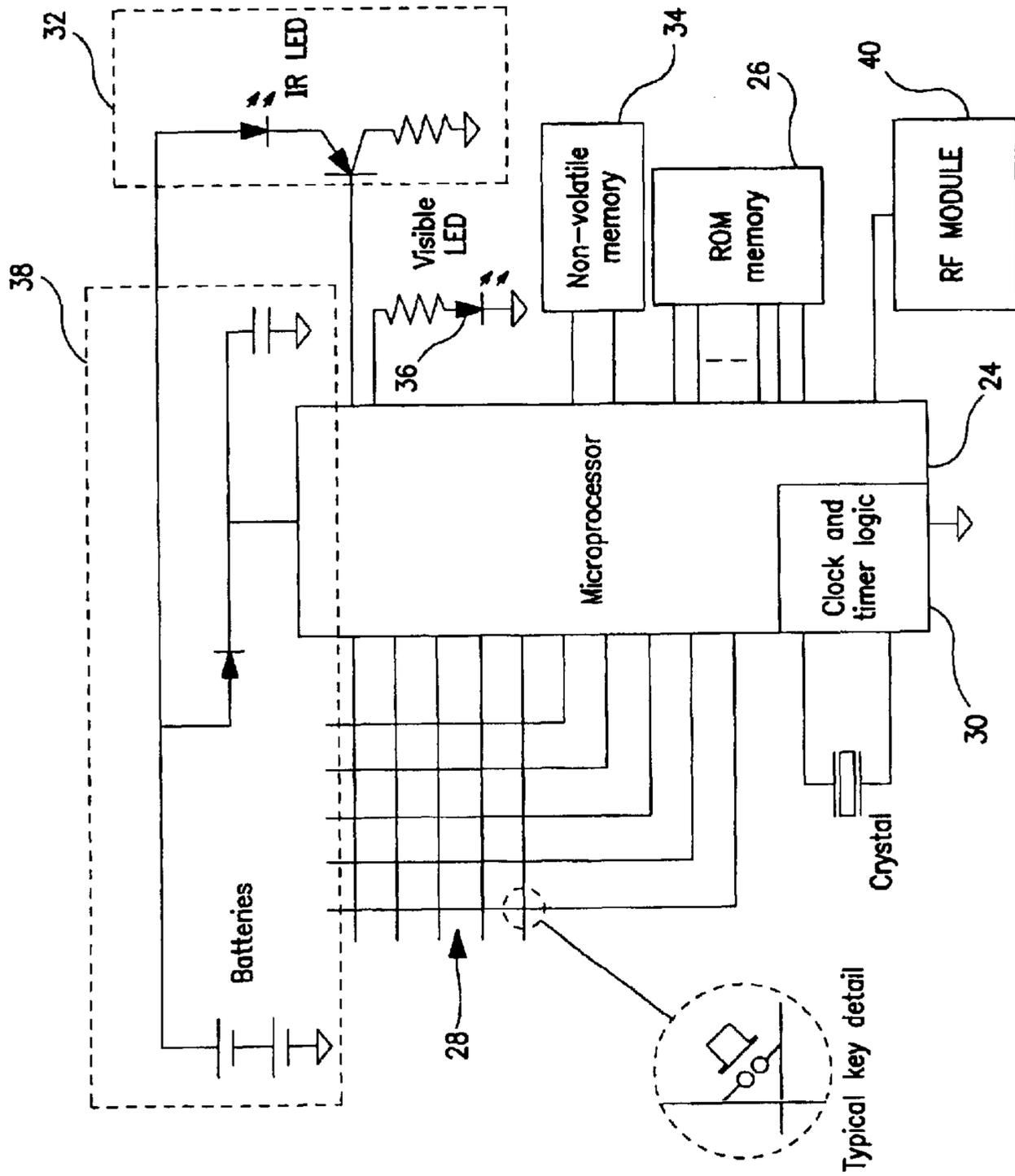
REMOTE CONTROL HARDWARE BLOCK DIAGRAM
