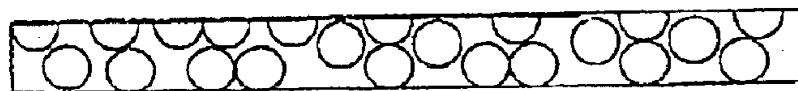
Figure 4. Paint film with cuprous oxide after some time in water. The paint film is partly eroded/polished.
