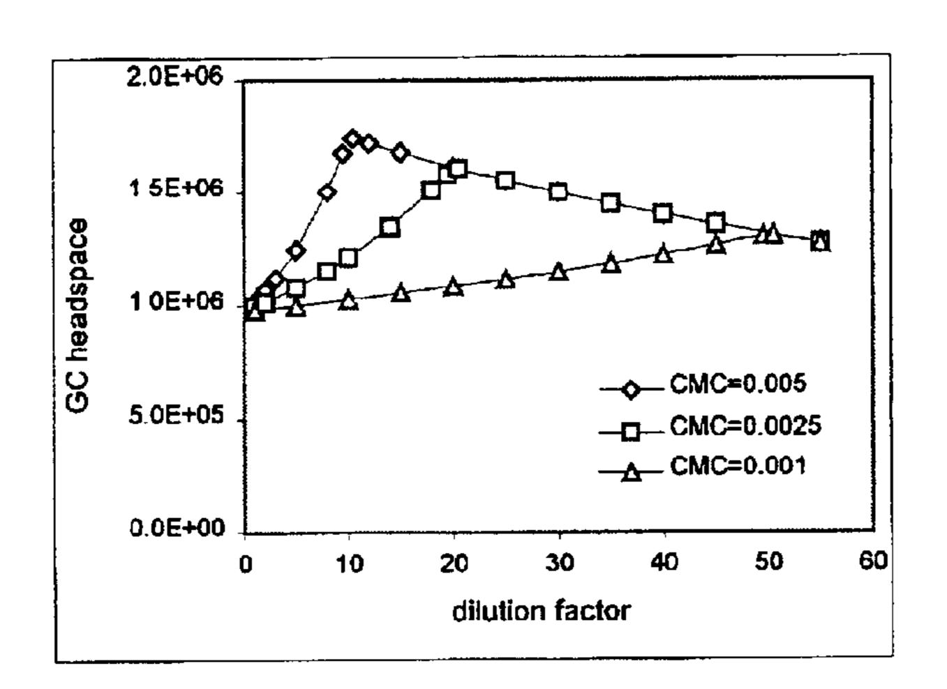
Figure 8: Experimental Results of Fragrance Burst with Change in CMC
