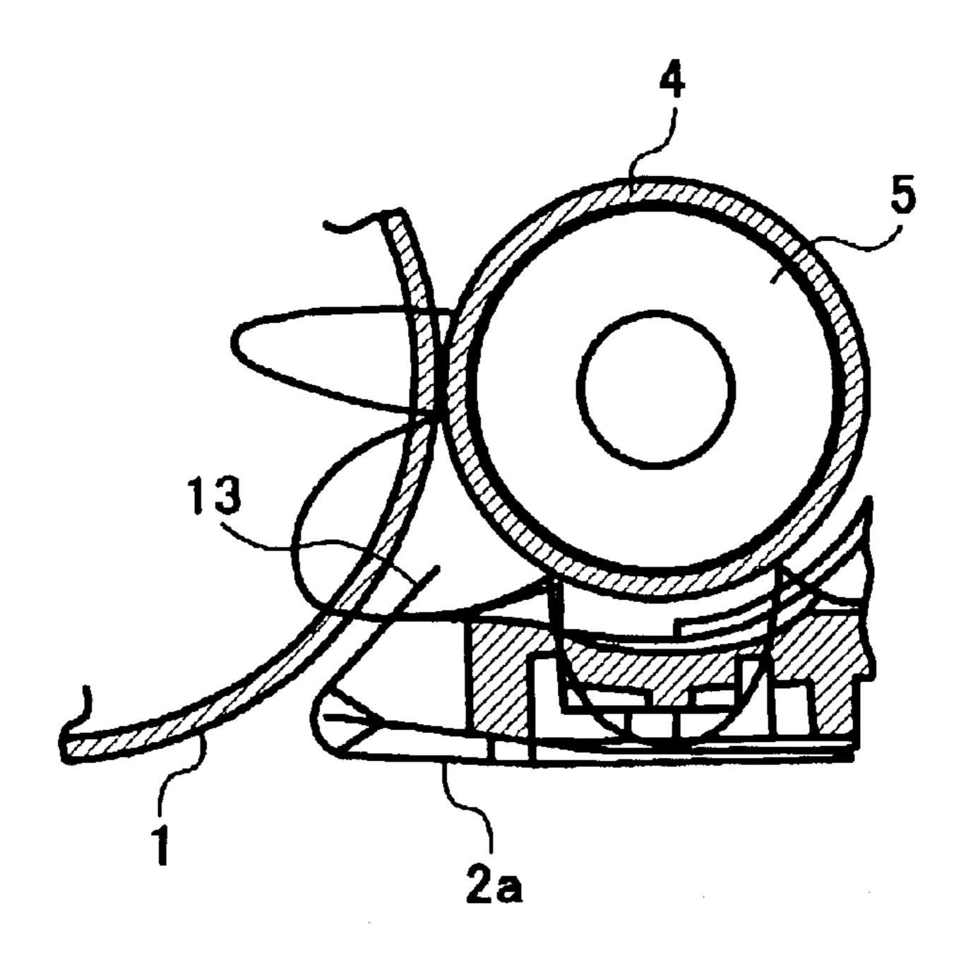
DEVELOPING DEVICE INCLUDING MAGNETIC MEMBER PROVIDED ON TONER-SCATTERING RESTRAINING DEVICE AND IMAGE FORMING APPARATUS INCLUDING THE DEVELOPING DEVICE
