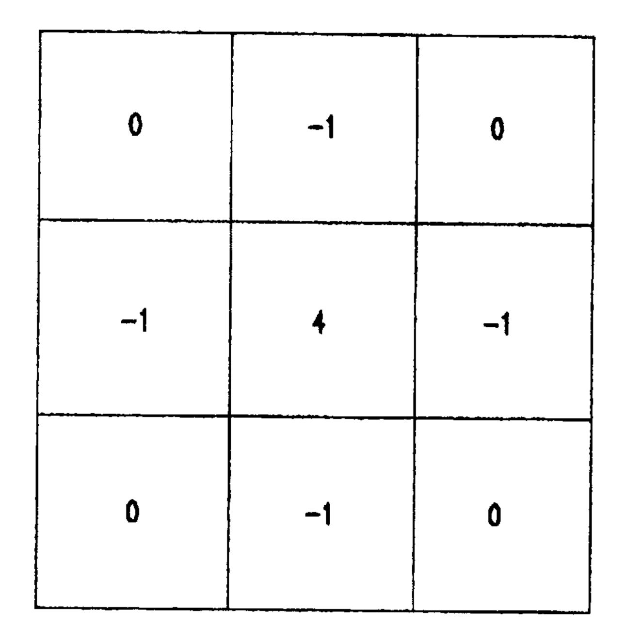
FIG. 6 LOW PASS FILTER COEFFICIENTS FOR BLURRING FUNCTION
