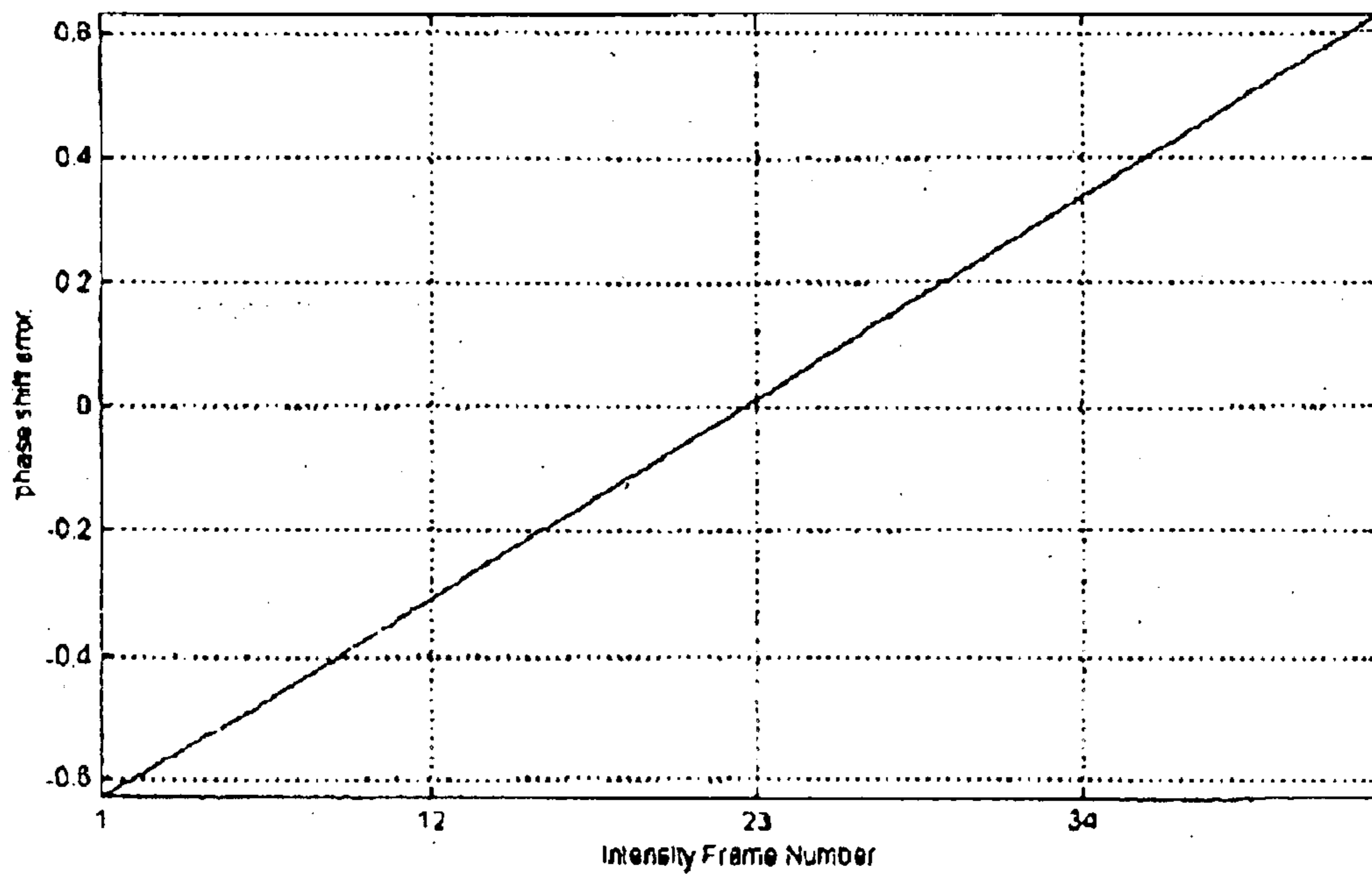
FIG 3 Phase shift error between adjacent interferograms
