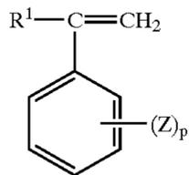
wherein R<sup>1</sup> is hydrogen, C<sub>1</sub>-C<sub>8</sub> alkyl, or halogen; Z is vinyl, halogen, or C<sub>1</sub>-C<sub>8</sub> alkyl; and p is 0 to 5.
