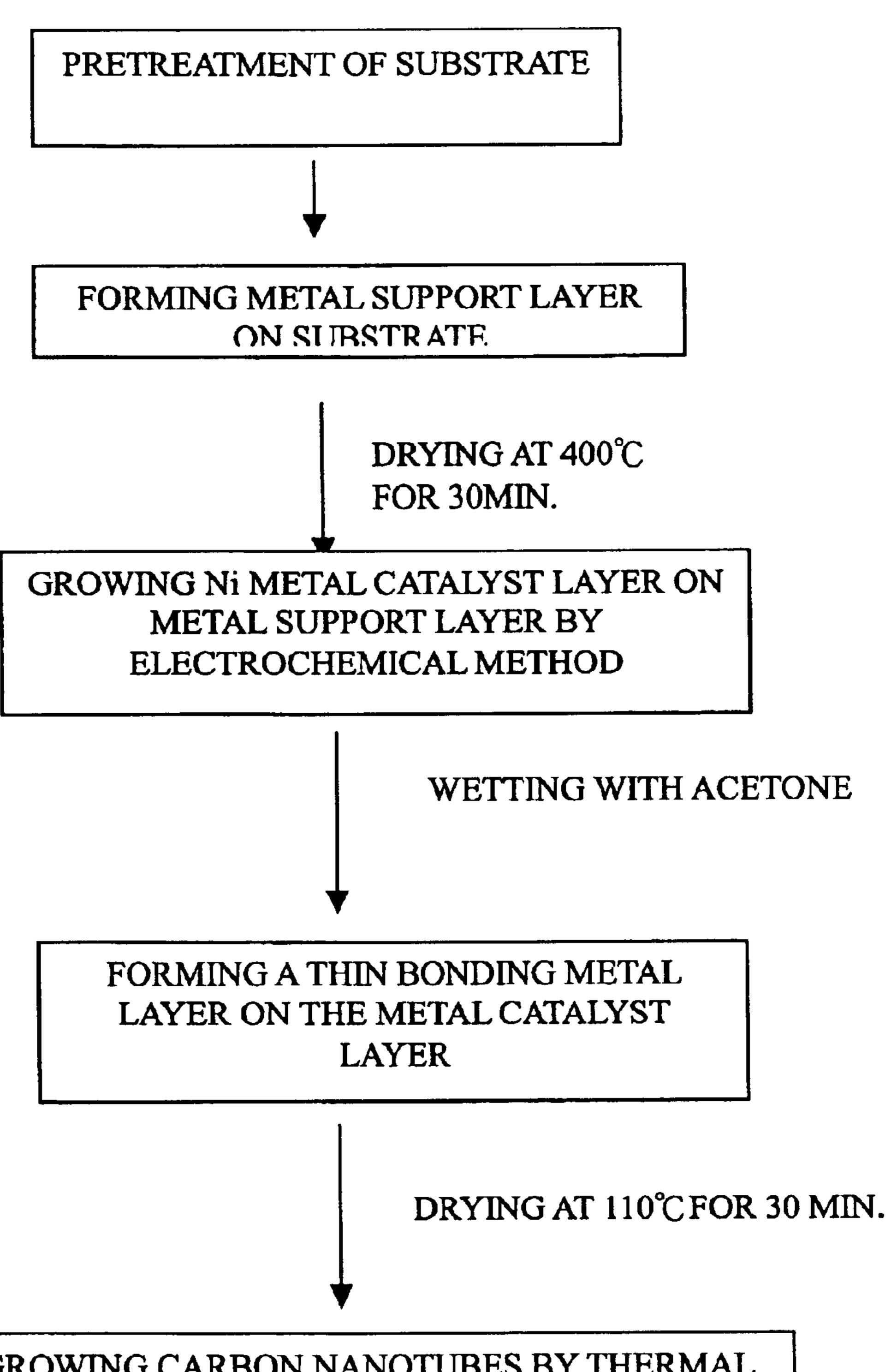
GROWING CARBON NANOTUBES BY THERMAL CVD AT LOW TEMPERATURE
