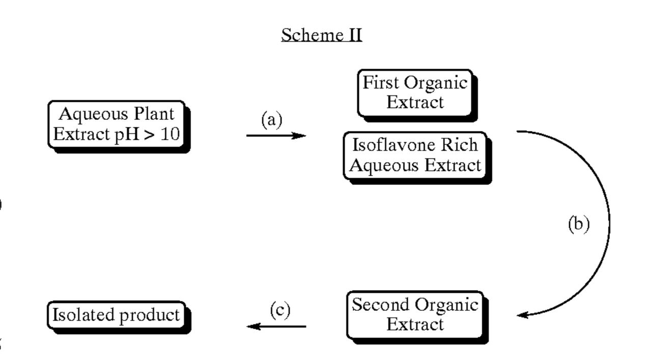
The pH of the starting aqueous plant extract can be elevated to greater than 10 and washed with an organic solvent as in step (a) from Scheme I to yield a first organic extract and an isoflavone rich aqueous extract. The resulting first organic extract contains impurities and is discarded. The isoflavone rich aqueous extract is then adjusted to an approximately neutral pH of 6–8 and extracted with an organic solvent as in step (c) from Scheme I to yield a second organic extract.
