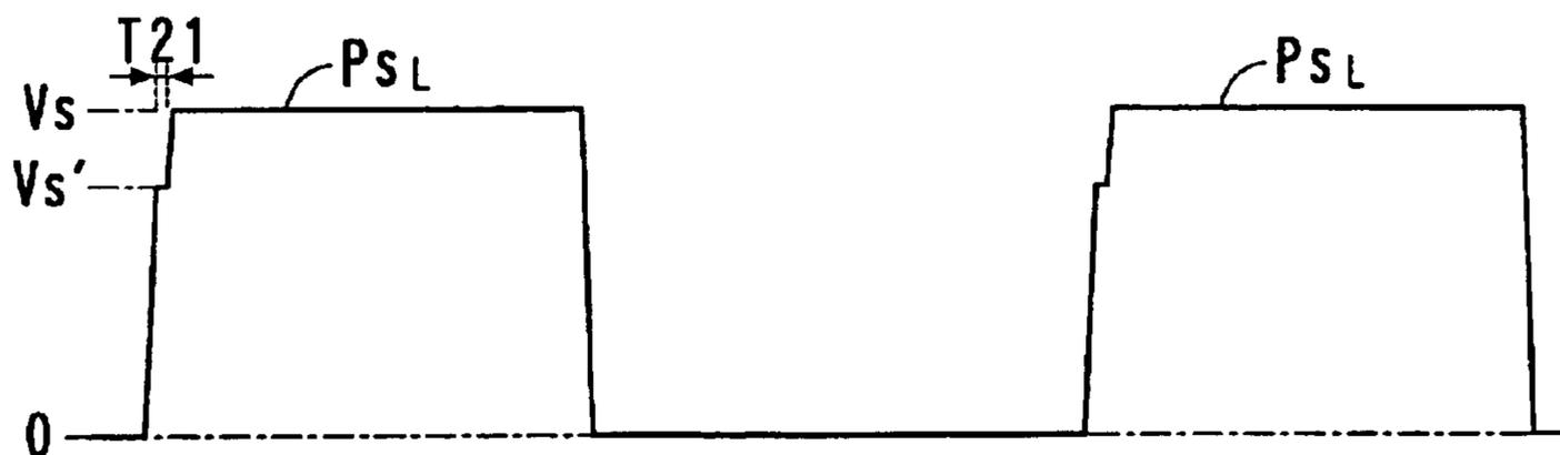
(B) WAVEFORM WHEN LIGHTING RATIO IS 41-60%
