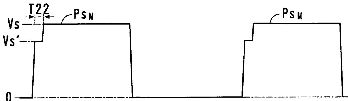
(C) WAVEFORM WHEN LIGHTING RATIO IS 61-100%
