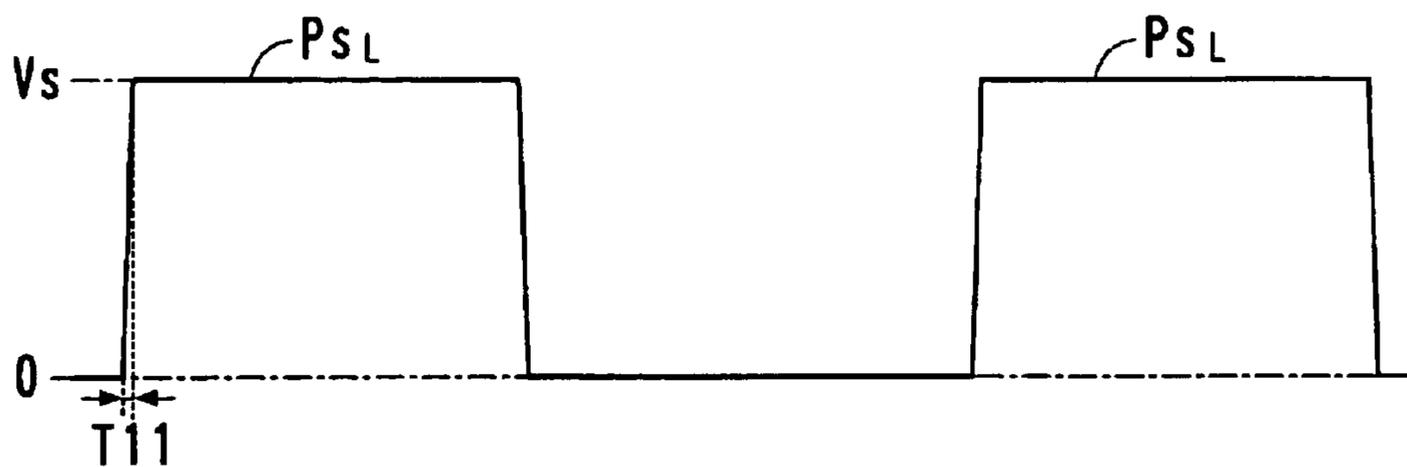
(B) WAVEFORM WHEN LIGHTING RATIO IS 41-60%
