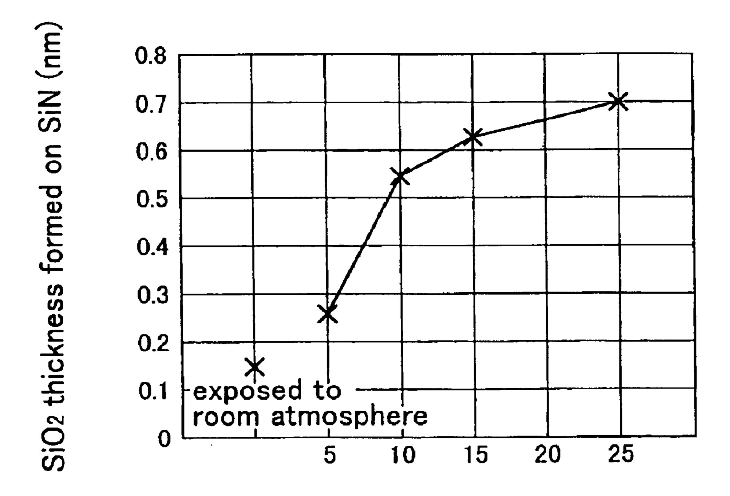
condition of wet oxidation as thickness of SiO2 formed on Si substrate (nm)
