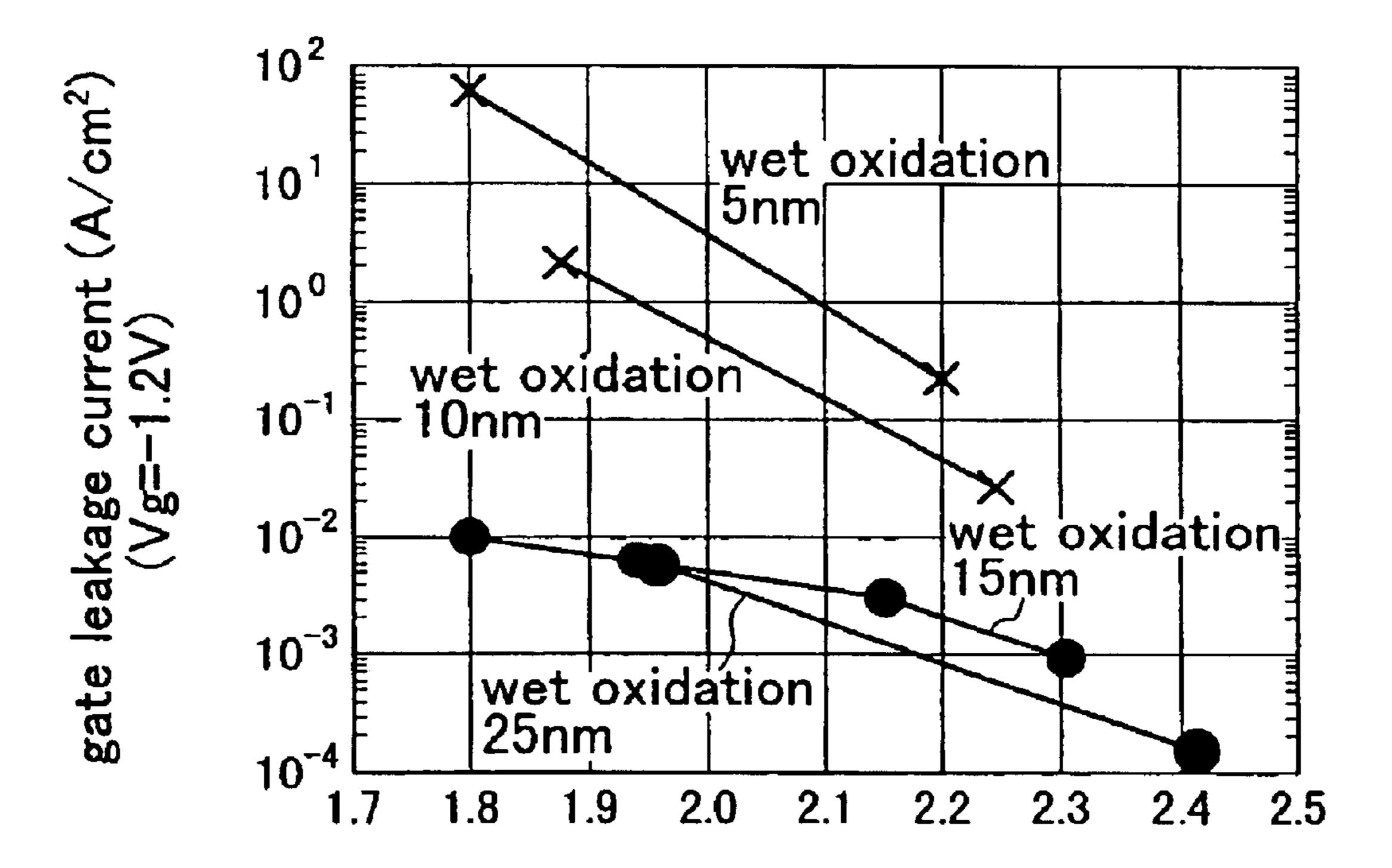
Equivalent oxide thickness (nm)
