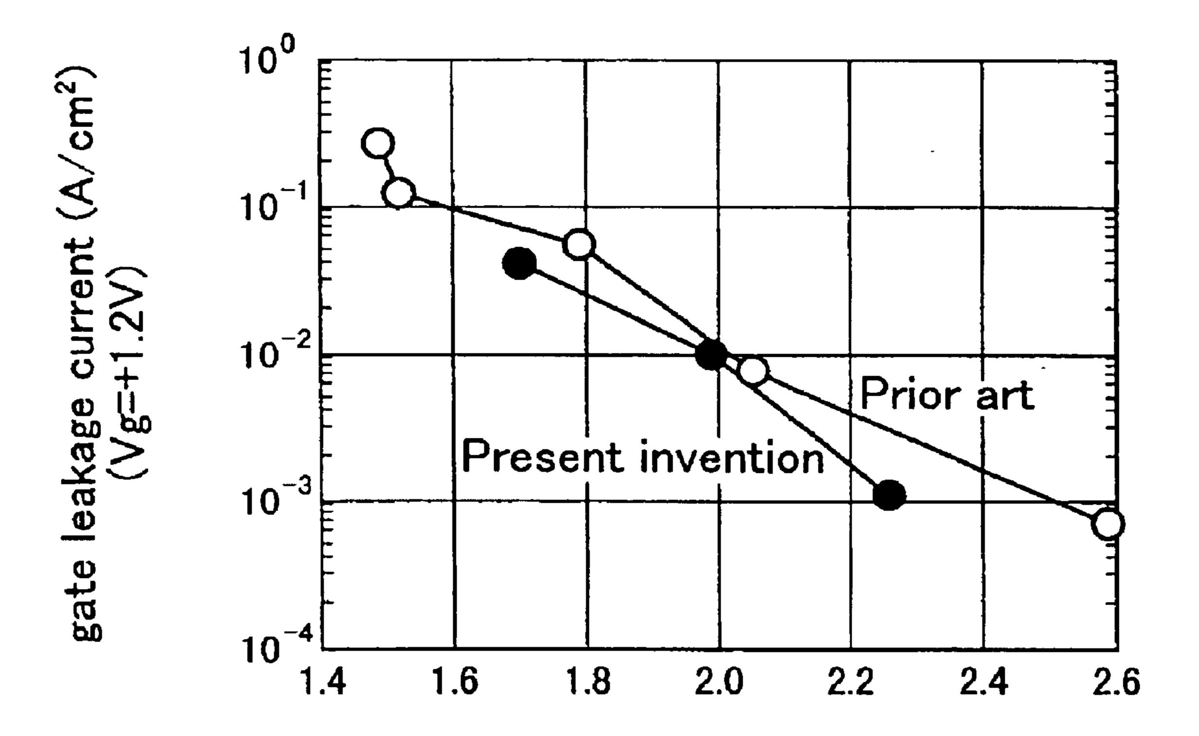
Equivalent oxide thickness (nm)
