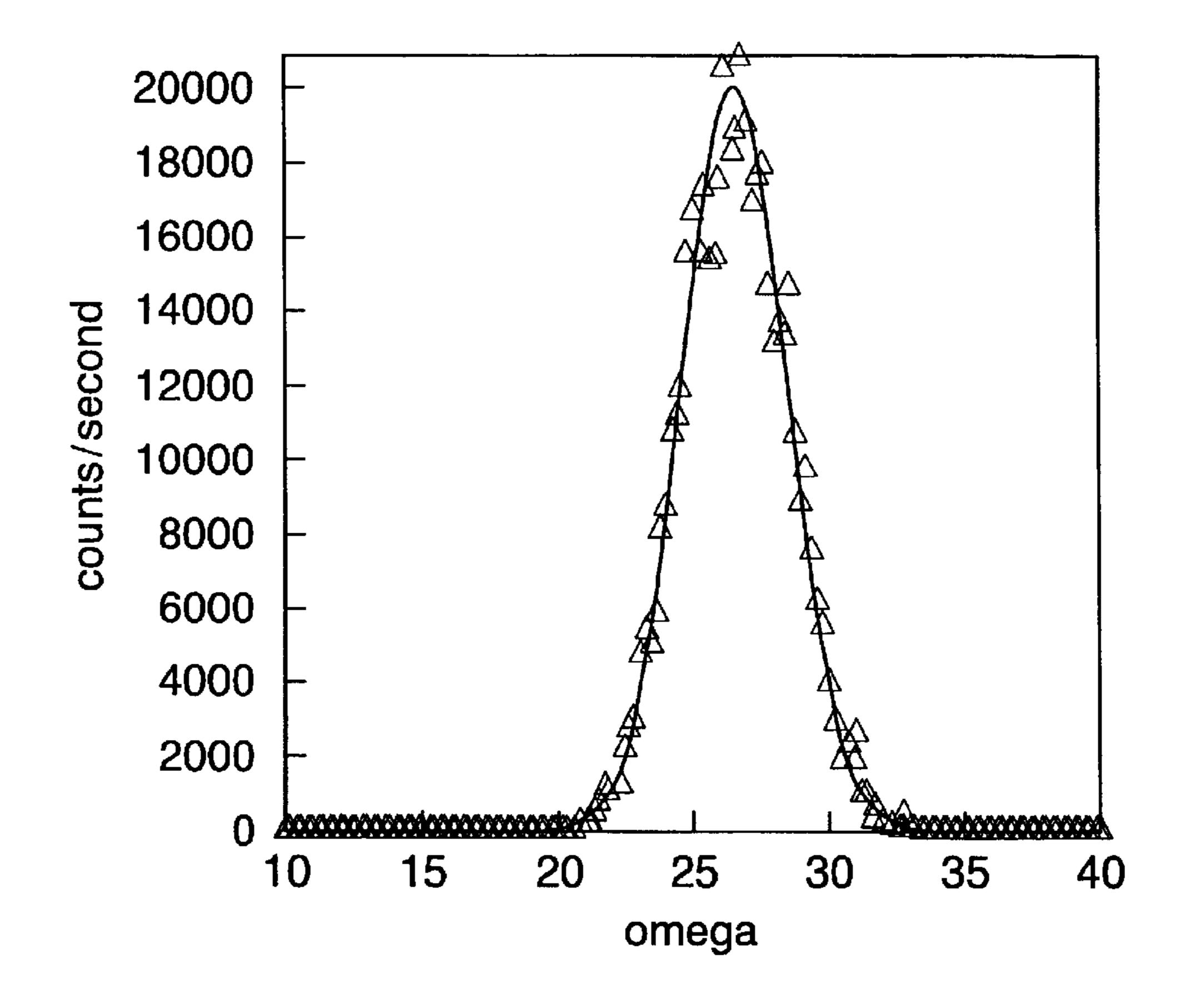
Ni-9at%W-0.03at%Mg alloy Annealing Temperature = 1400°C
