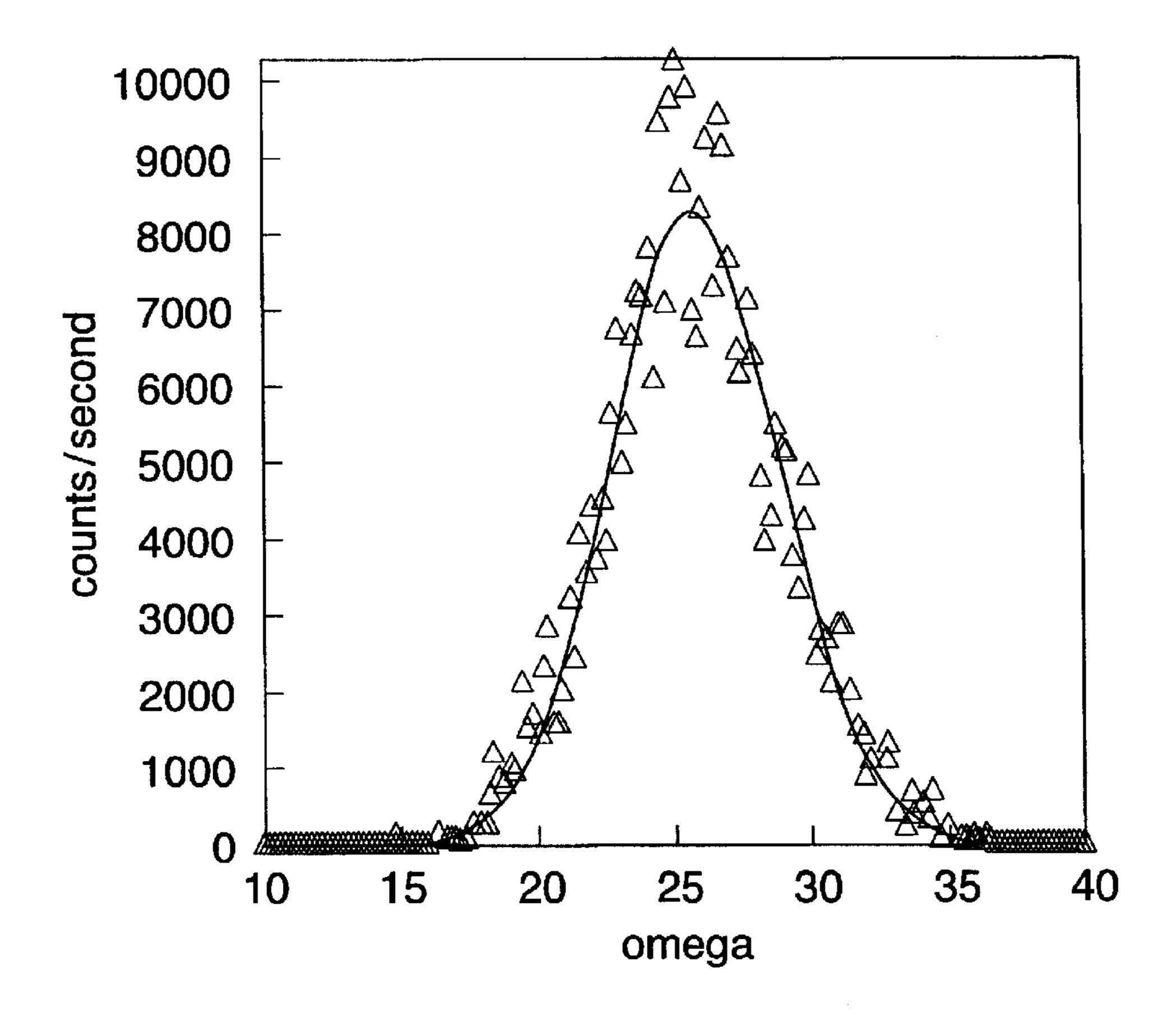
Ni-13at%Cr-0.03at%Mg alloy Annealing Temperature = 1400°C
