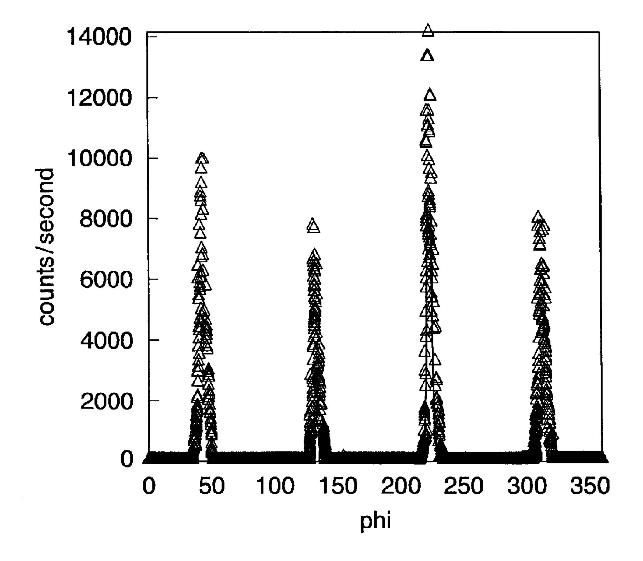
Ni-9at%W alloy Annealing Temperature = 1400°C
