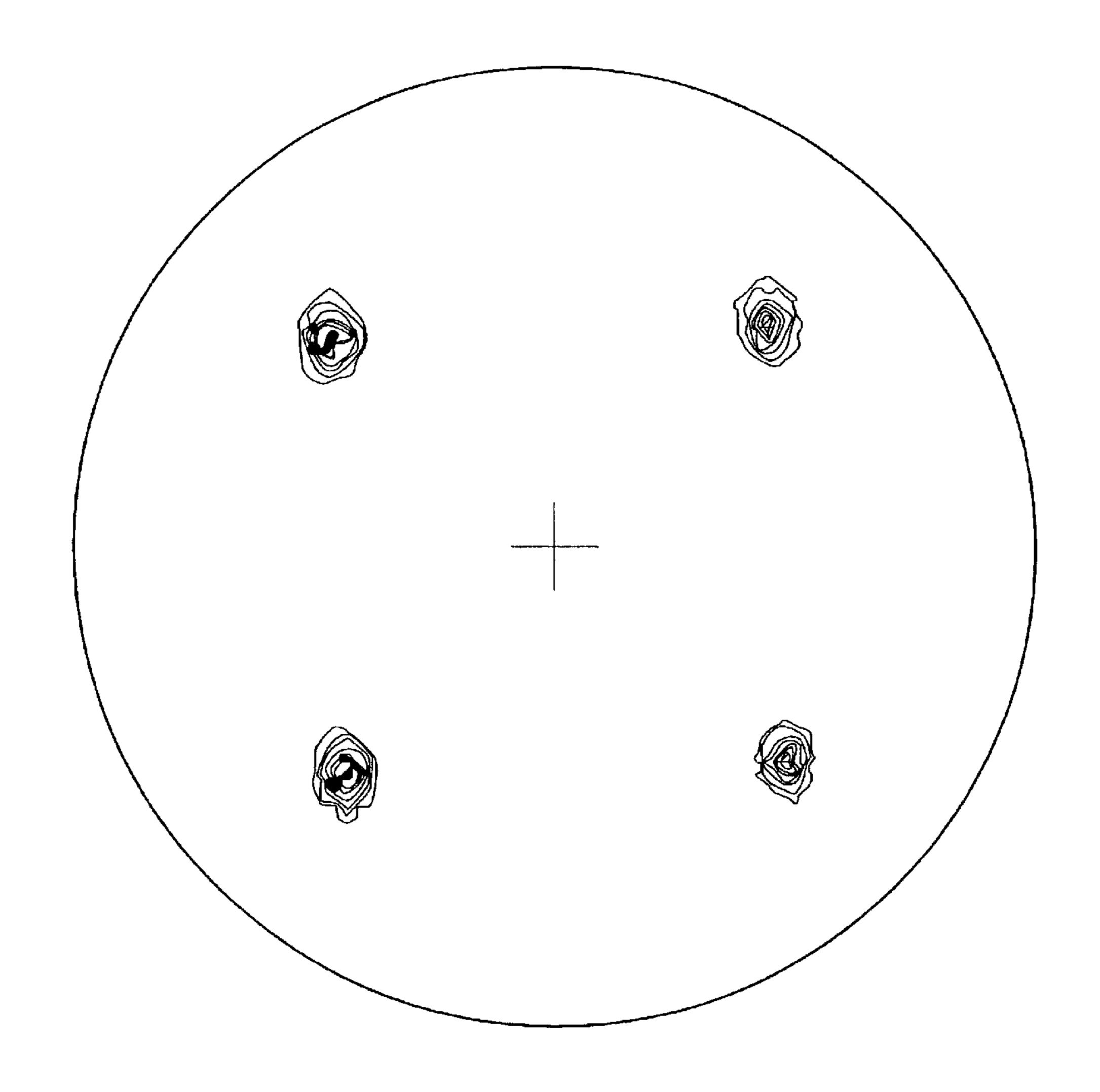
Ni-9at%W alloy Annealing Temperature = 1200°C
