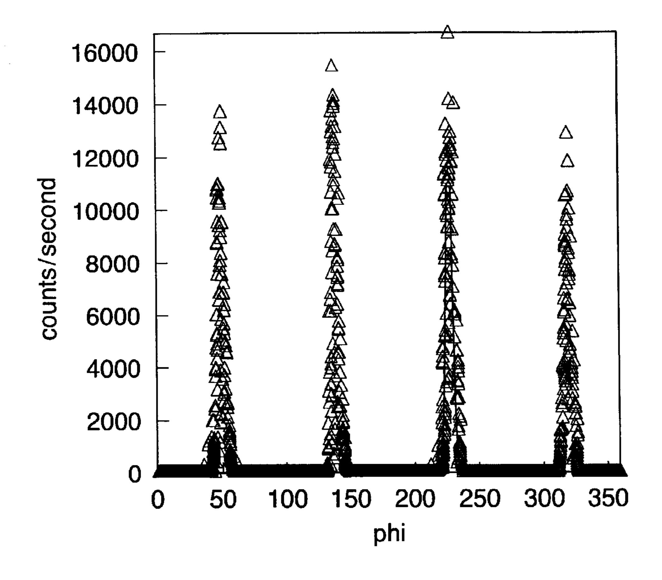
Ni-9at%W-0.03at%Mg alloy Annealing Temperature = 1400°C
