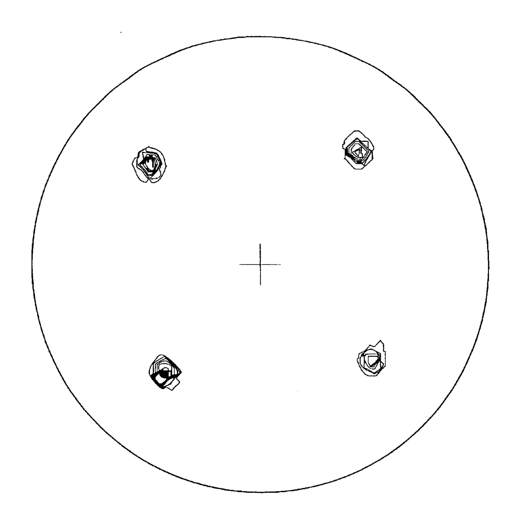
Ni-9at%W-0.03at%Mg alloy Annealing Temperature = 1400°C
