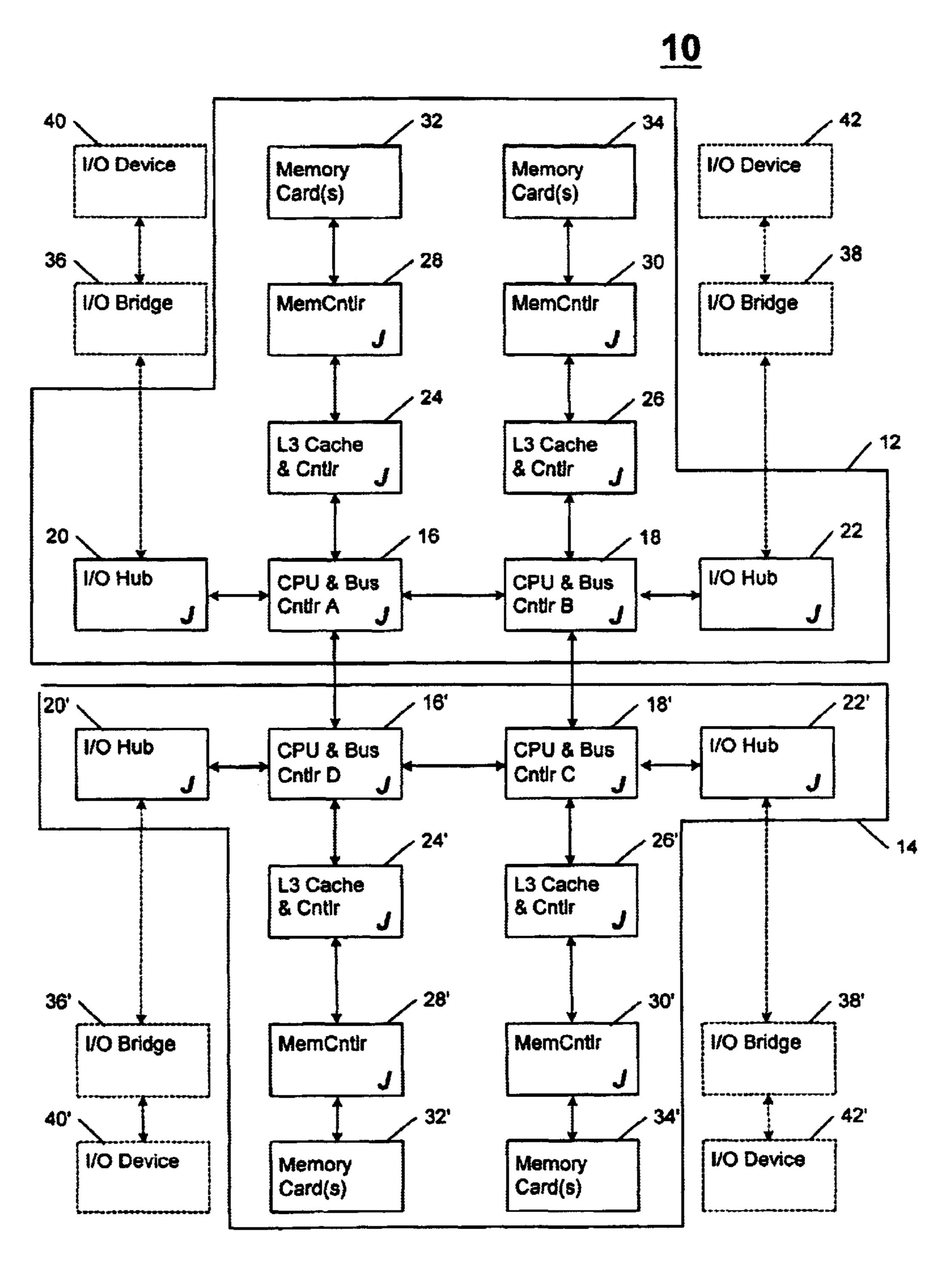
J = chip has serial jtag connection to Service Processor HW
