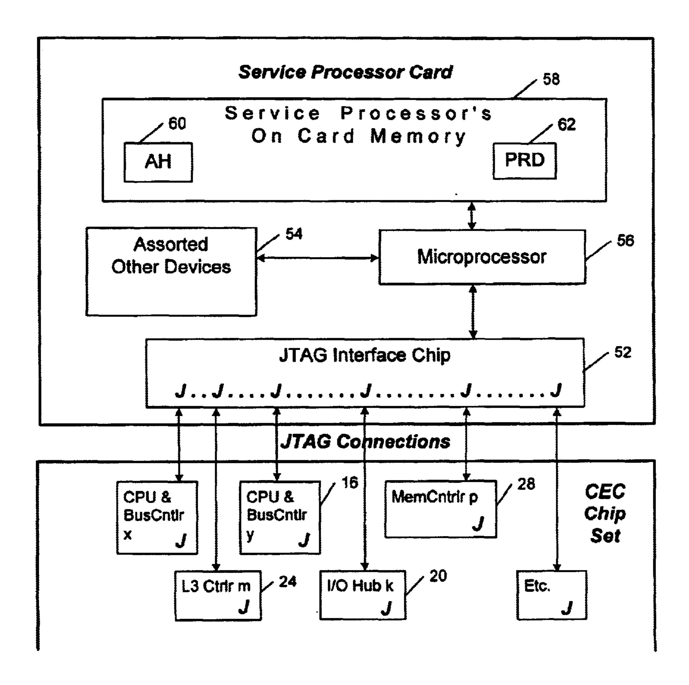
J = JTAG serial interface between Service Processor & chips in CEC
