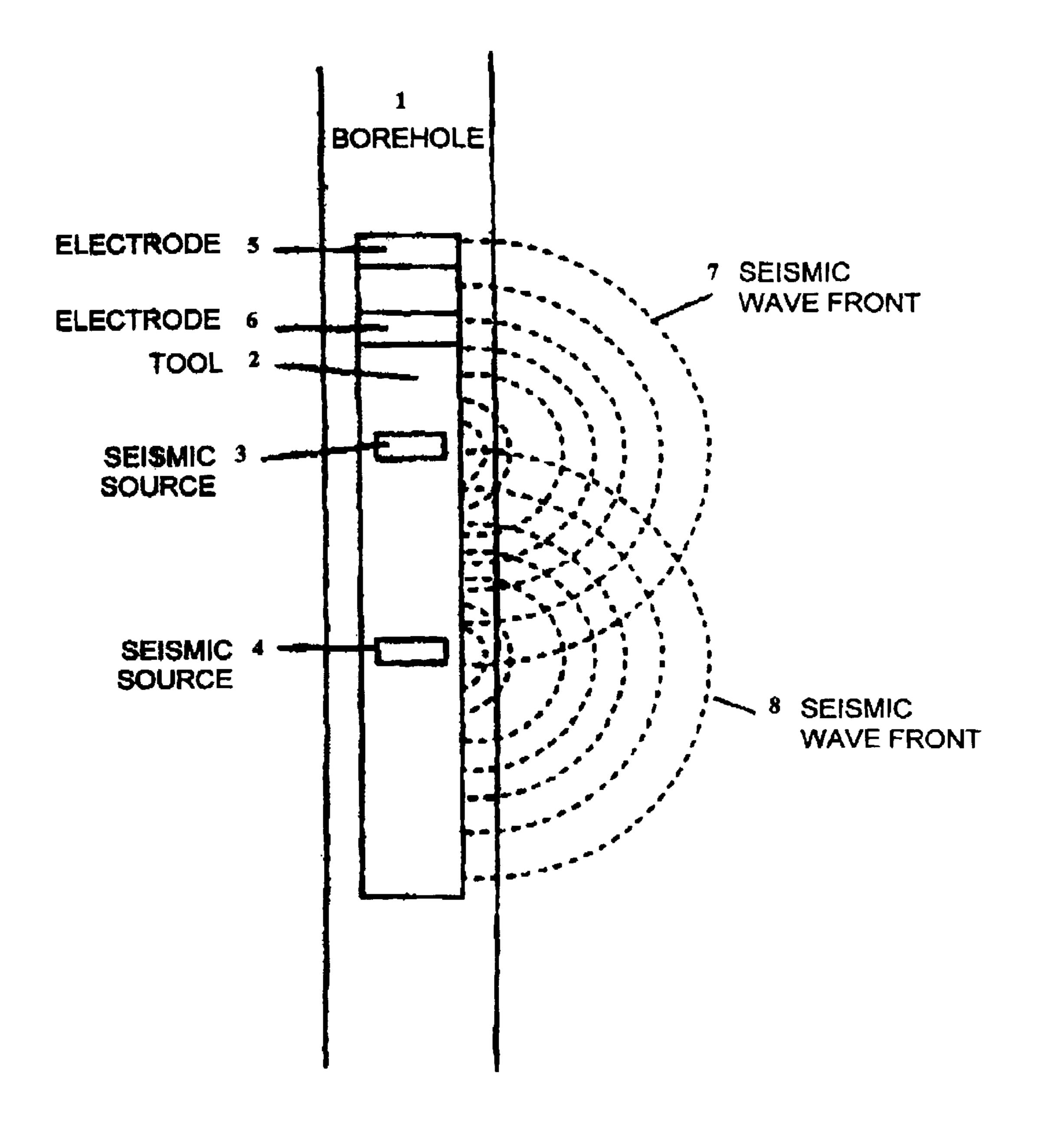
The present invention relates to a method and equipment for measuring the properties of subsurface rock from a tool
