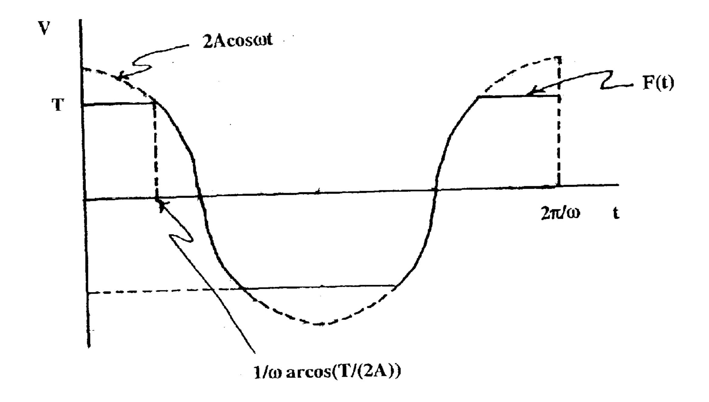
$F(t) = a_0/2 + \sum_{n=1}^{\infty} a_n cosn\omega t, \text{ where } a_n = (2\omega/\pi) \int_{\sigma}^{\overline{\nu}/\omega} F(t) cosn\omega t dt. \text{ In particular,}$   $a_1 = (8A/\pi)\{(T/(4A^2))[4A^2 - T^2]^{1/2} + \pi/4 - (1/2)arcos(T/(2A)) - (1/(4A))[4A^2 - T^2]^{1/2}\}.$  If T = 1.186 A, this formula yields  $a_1 = A$ , i.e., if  $2A\cos\omega t$  is truncated at +/-1.186 A, the frequency  $\omega$  component of the truncated waveform has amplitude A.
