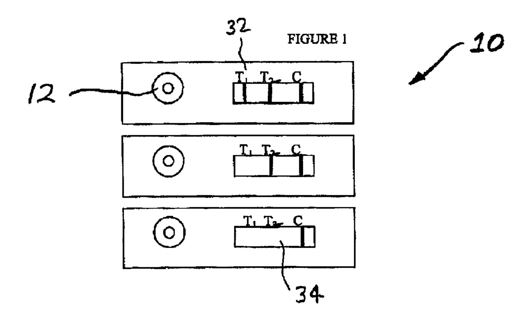
Sample is added to well at left and flow is from left to right.
