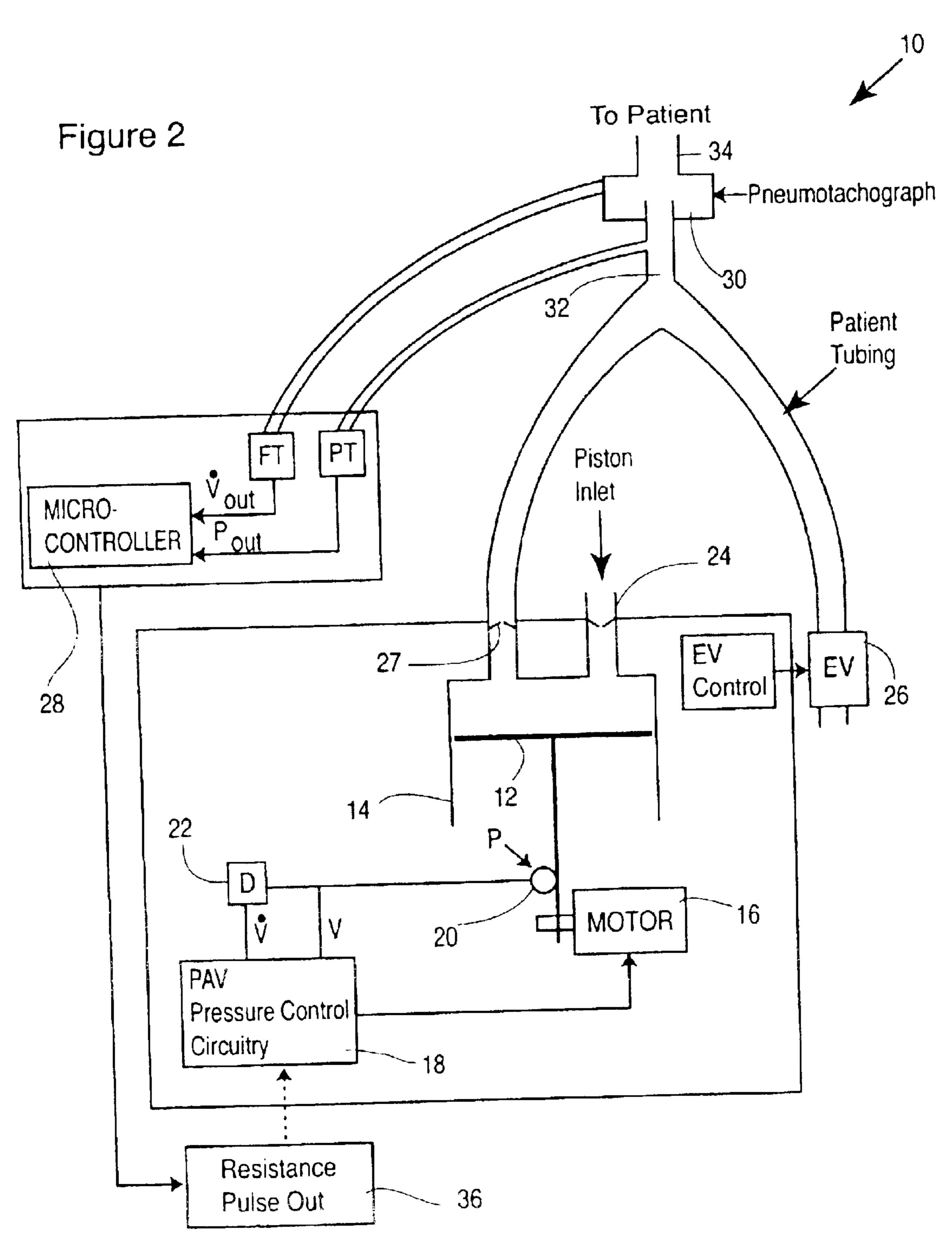
D = Differentiator; EV = Exhalation Value; P = Potentiometer;  $P_{out}$  = Airway Pressure Signal; V = Volume Sig
