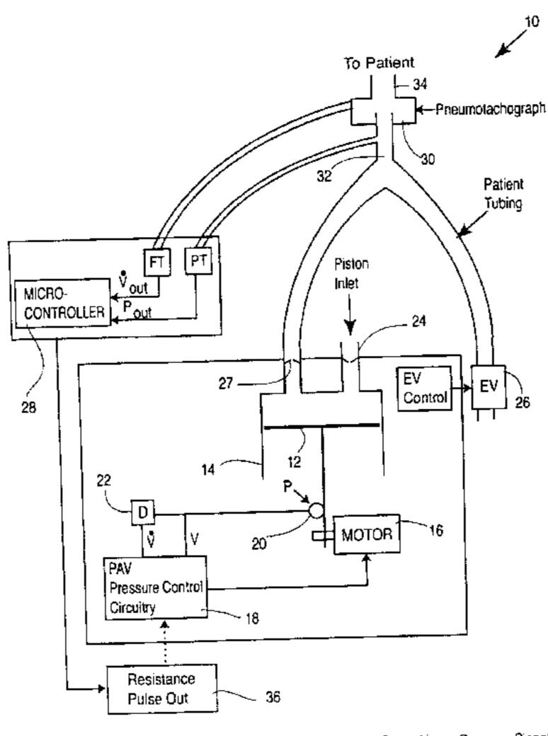
D = Differentiator; EV = Exhalation Value; P = Potentiometer;  $P_{out}$  = Airway Pressure Signal; V = Votume Signal;  $\tilde{V} = Flow Signal$ ;  $\tilde{V}_{out} = Flow Signal Output Port$
