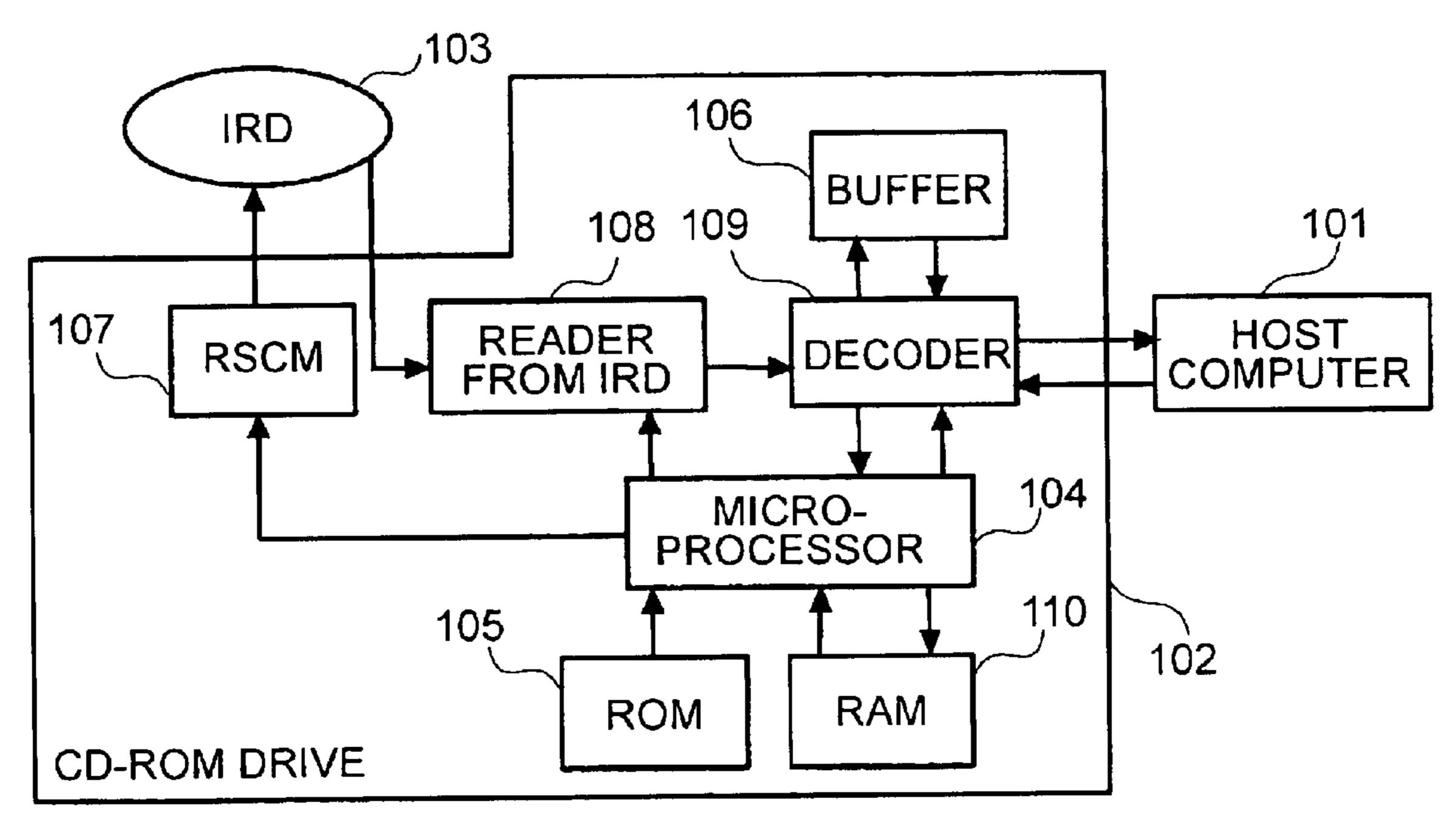
IRD:Information Recording Disk RSCM:Revolving Speed Control Means
