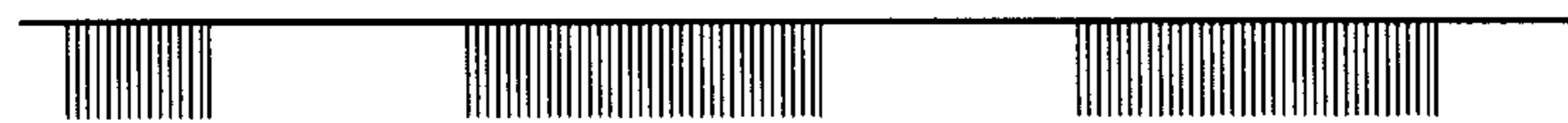
Modulated signal for code 0100100111
