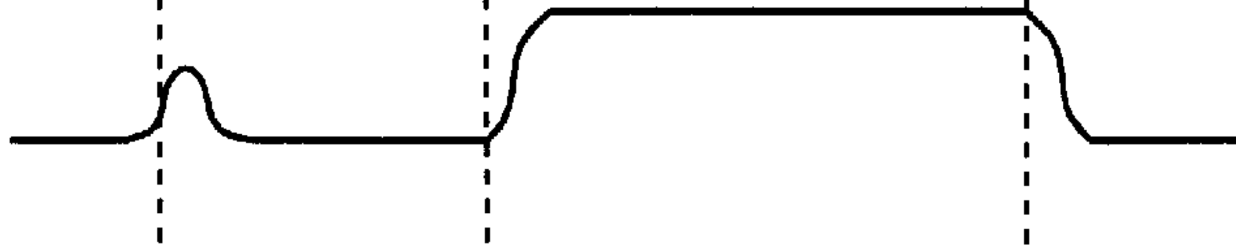
FIG. 6B LUMINANCE DISTRIBUTION DETERIORATED BY APERTURE EFFECT
