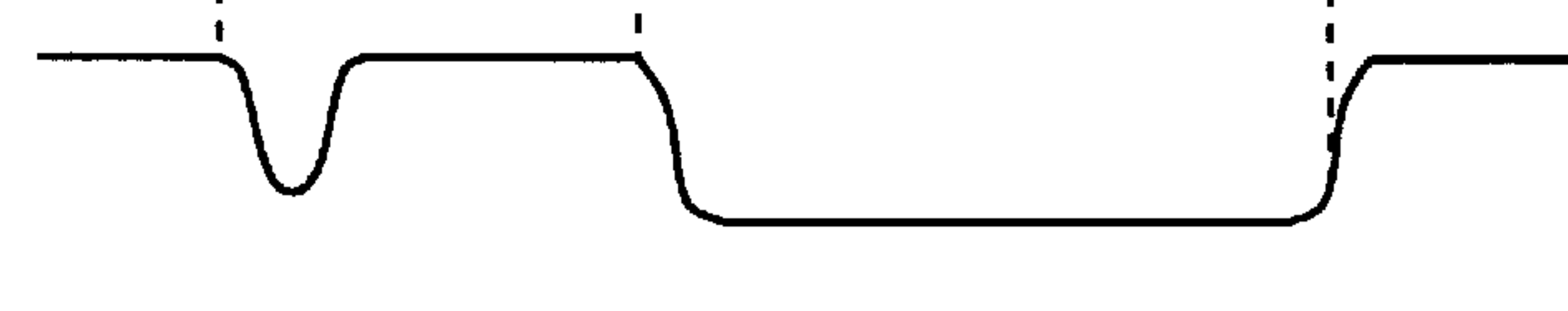
FIG. 7D LUMINANCE DISTRIBUTION IMPROVED BY APERTURE CORRECTION
