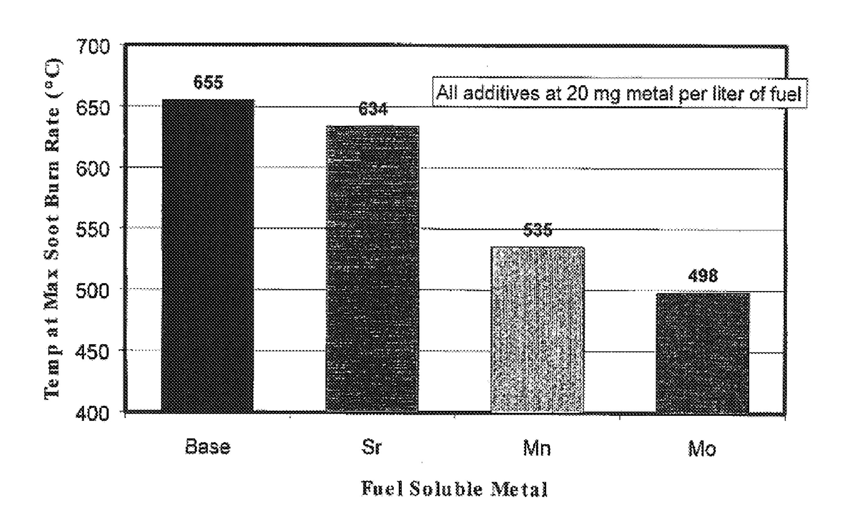
Figure 2: Metal Gravimetric Efficiency in Soot Light-Off
