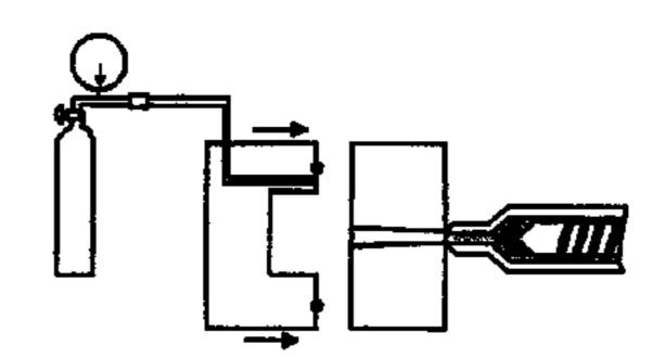
2. Injection into the cavity under counter-pressure
