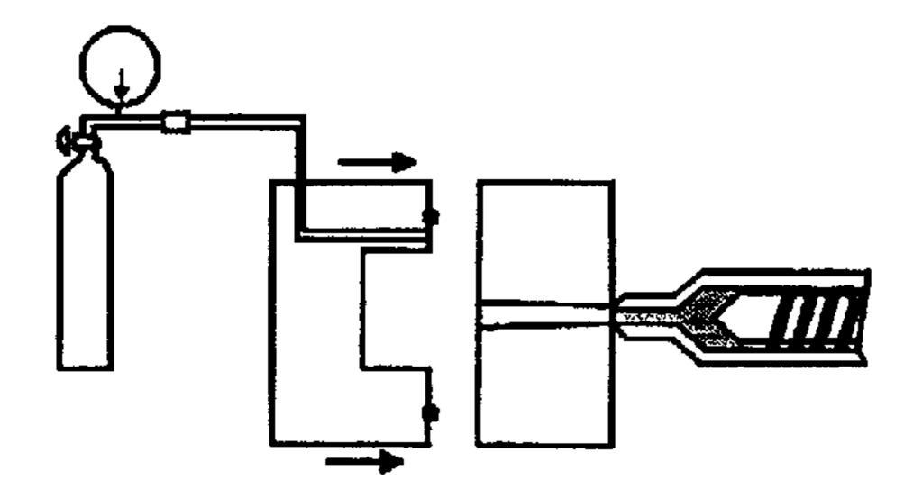
2. Injection into the cavity under counter-pressure
