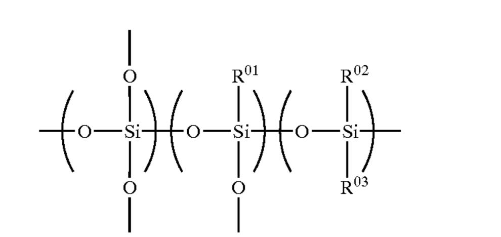
A siloxane-derived resin having the above-described formula (IV) is formed by sol-gel conversion from a dispersion comprising at least one kind of silane compound(s) represented by the following formula (V). In formula (IV), at least one of R<sup>01</sup> to R<sup>03</sup> represents a hydroxyl group, the other groups represent organic residues selected from R<sup>0</sup> and Y in the following formula (IV).
