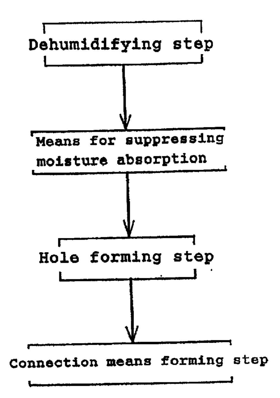
(C)Dehumidifying step Means for suppressing moisture absorption Hole forming step Connection means forming step
