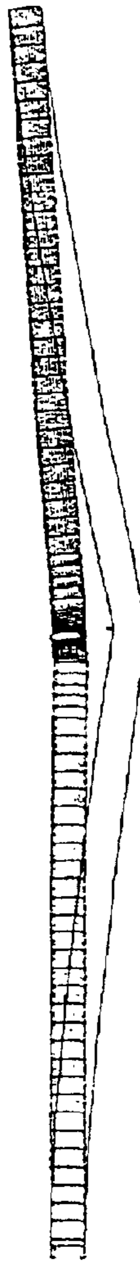
Pipeline Wrinkle - 12.75 in - 500 pct. w.t. - l/h = 3 - 270 deg.
