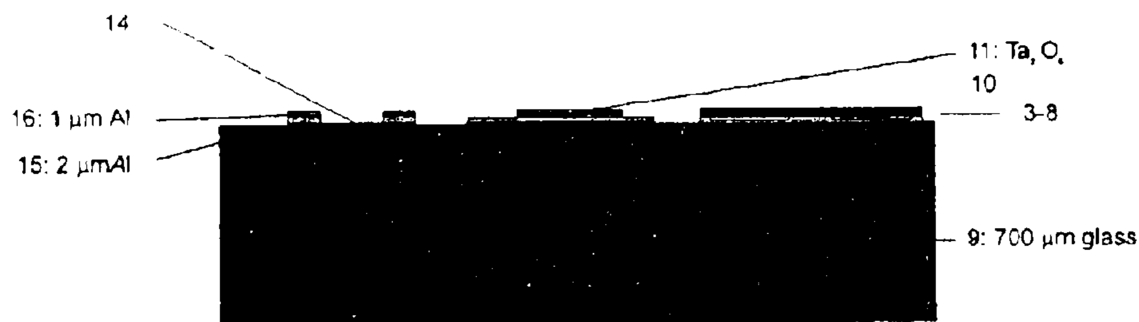
Figure 3c: Integration of the TaN (14) resistors and Ta (11-10) capacitors. The HEMT device is protected by the bottom Al layer (15) during the processing.
