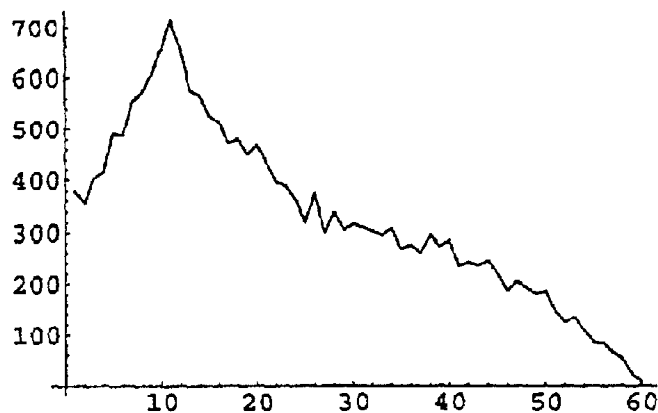
Figure 3. Spectrum of Twice Compton Scattered Gammas from 140 keV Source - Energy Range 80-140 keV
