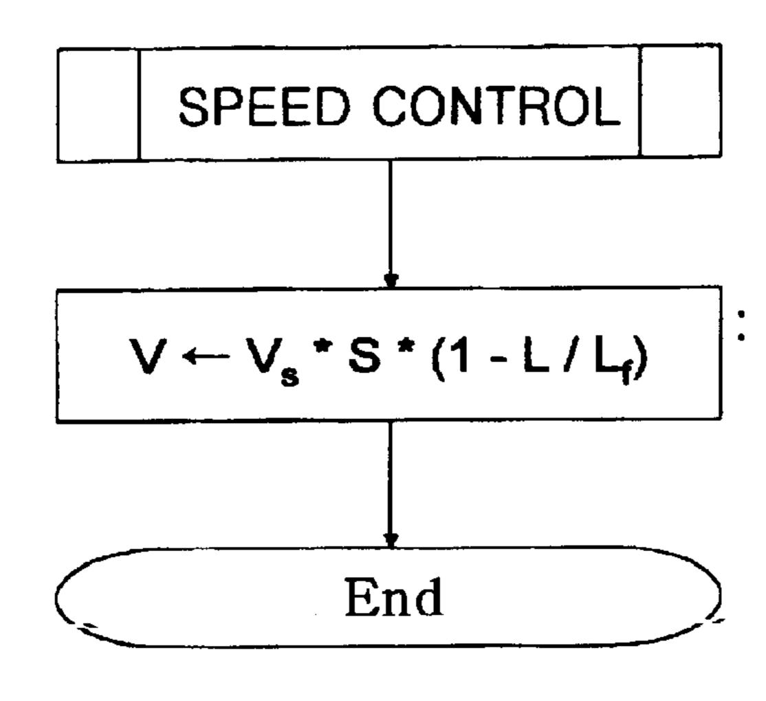
: Speed Control by comparing the amount of winding with L<sub>f</sub>
