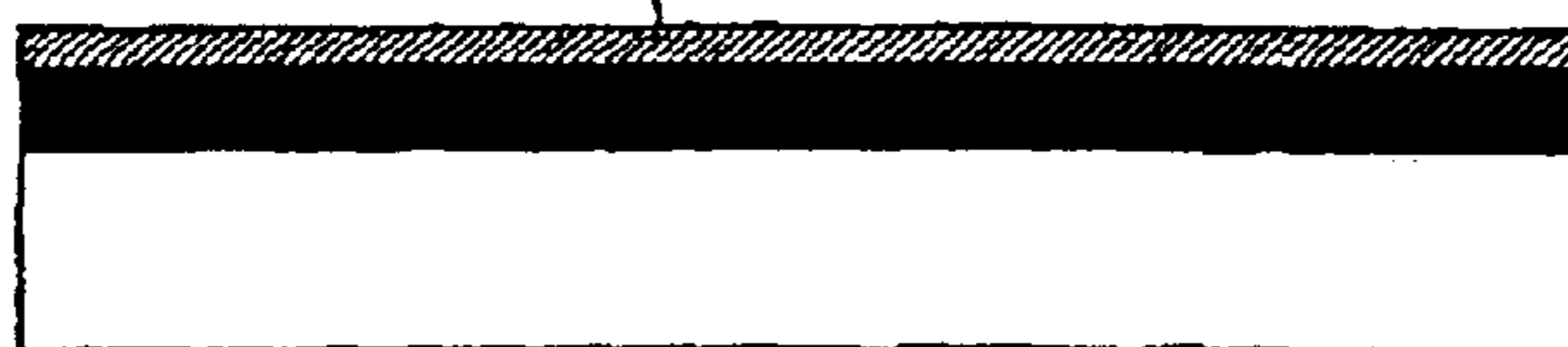
(B) Al deposition (evaporation or sputtering)
