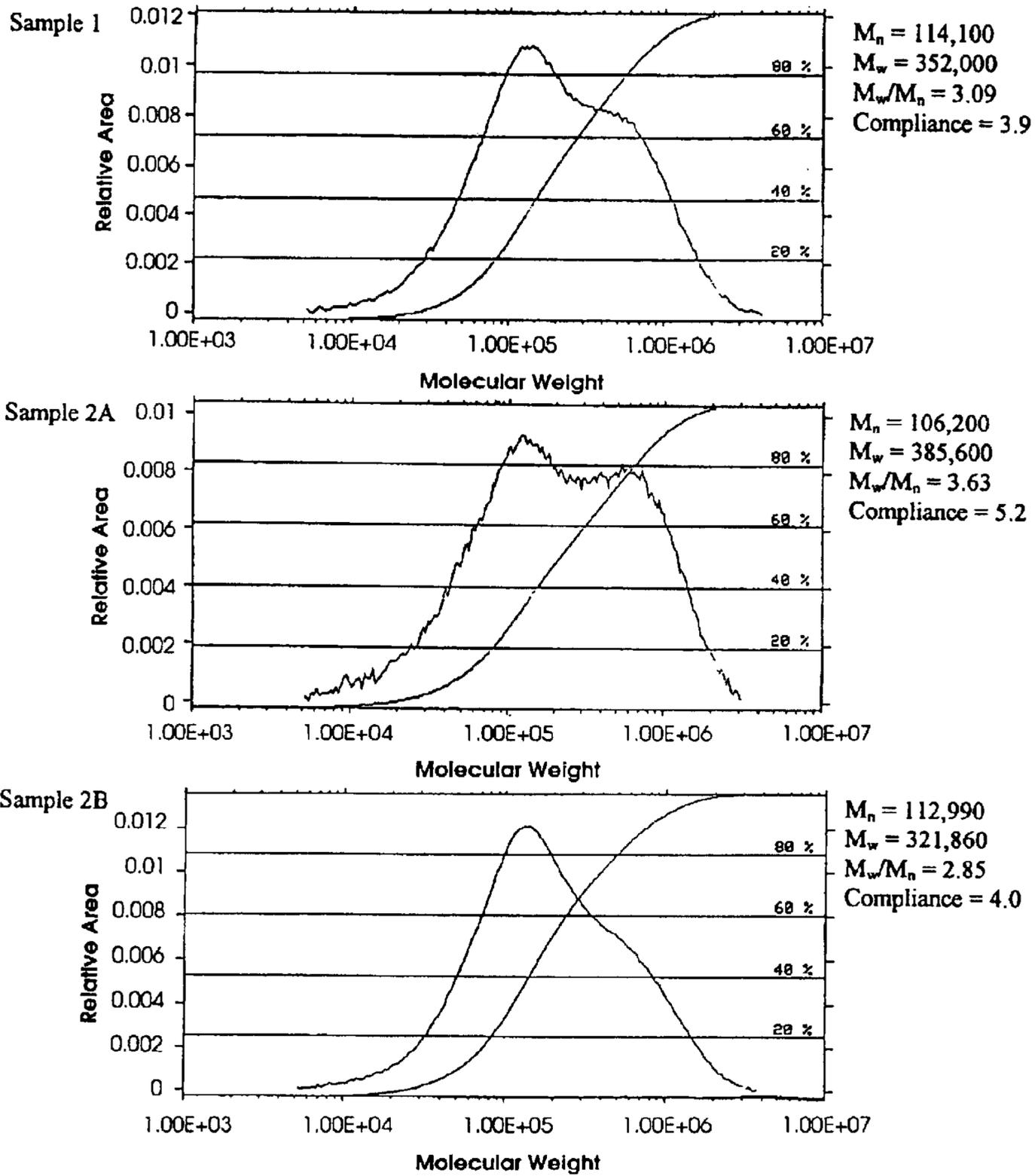
\*GPC plots are of Relative Area versus Molecular Weight. Recoverable Compliance numbers track the high end of the distribution and are in units of  $\text{Pa}^{-1} \times 10^{-4}$ . Compliance is measured at about 200°C per Exxon test method.
