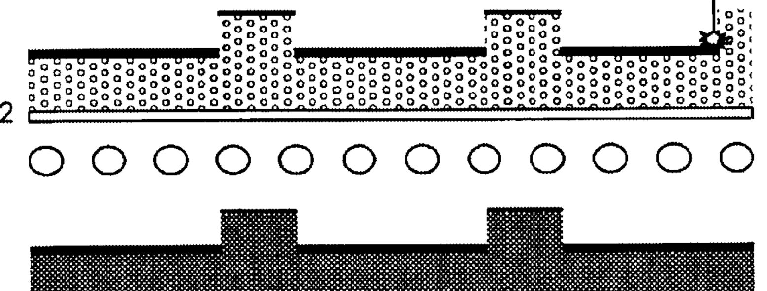
IR Laser "collapsing" microspheres to create relief.
