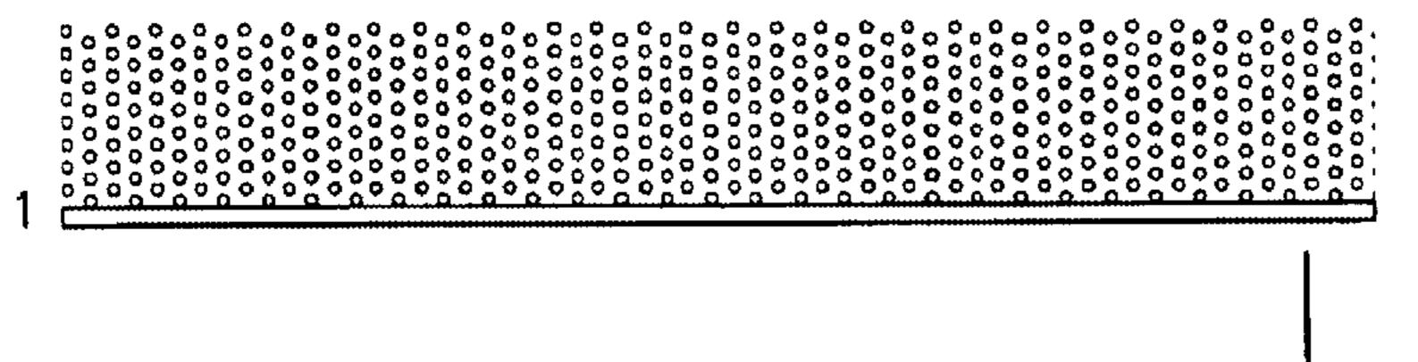
Raw UV curable plate material, with IR sensitive microspheres.
