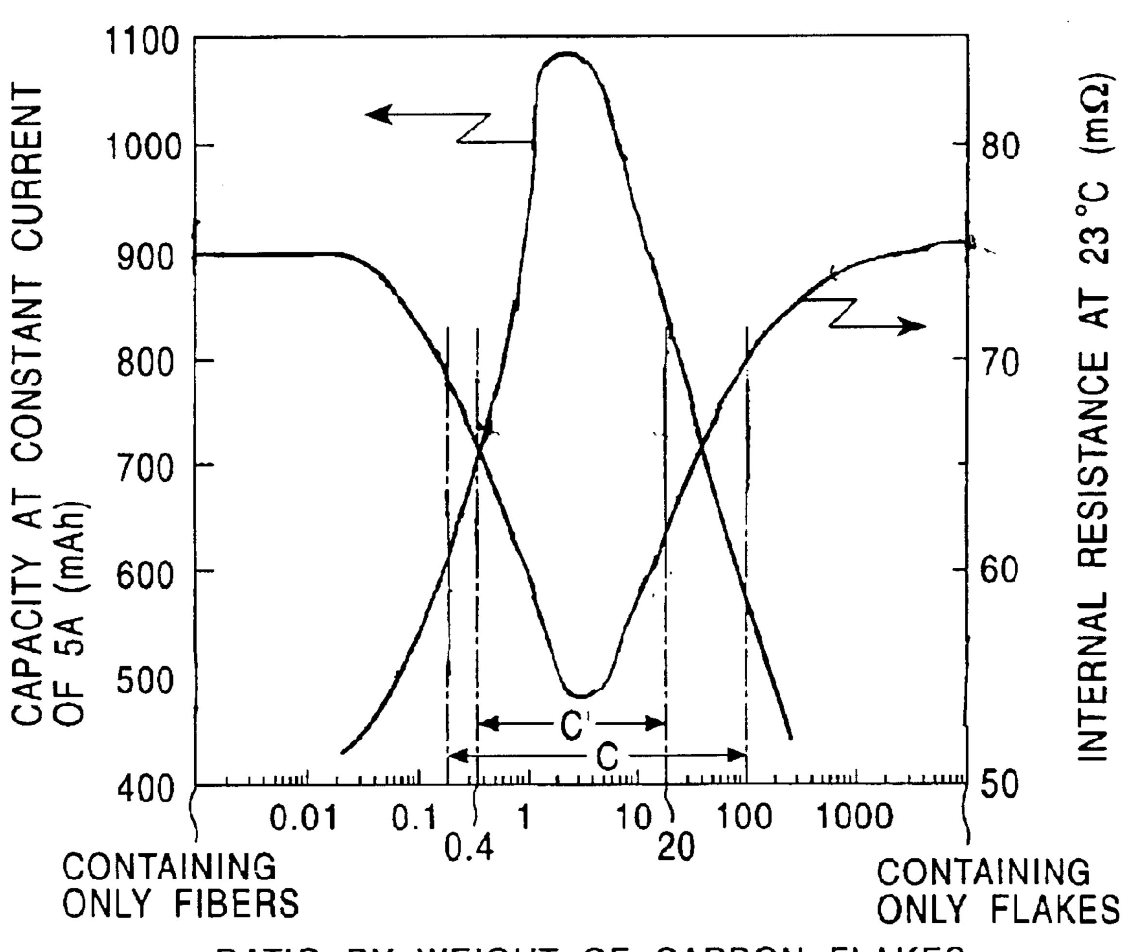
RATIO BY WEIGHT OF CARBON FLAKES KS-15 TO CARBON FIBERS VGCF
