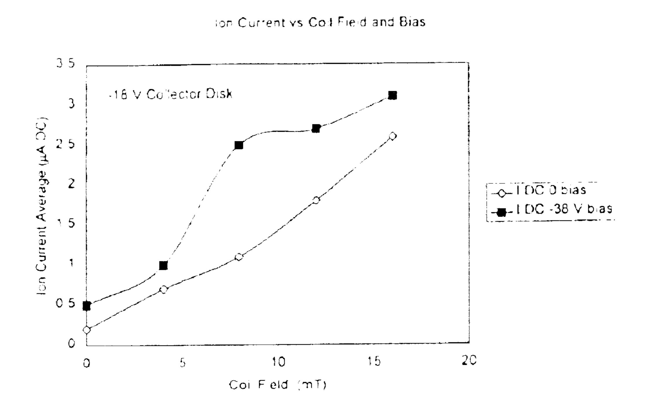
Fig. 5 shows the collector current for the second embodiment of the invention as a function of the deflection tube magnetic field level and deflection plate bias level
