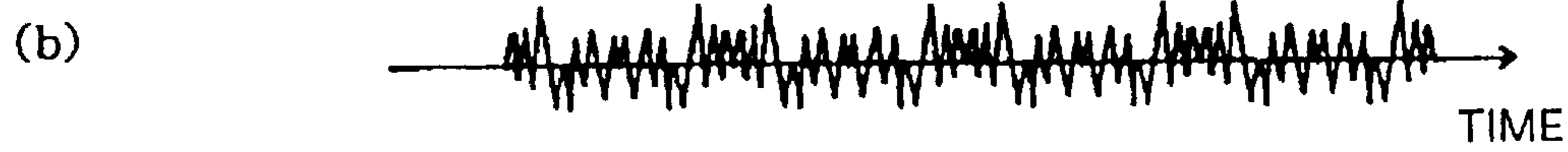
CORRELATED VALUES = INTERFERENCE LEVEL UPON RECEPTION OF BROADCASTING CHANNEL WITH SPREADING CODE FOR INDIVIDUAL DATA CHANNEL
