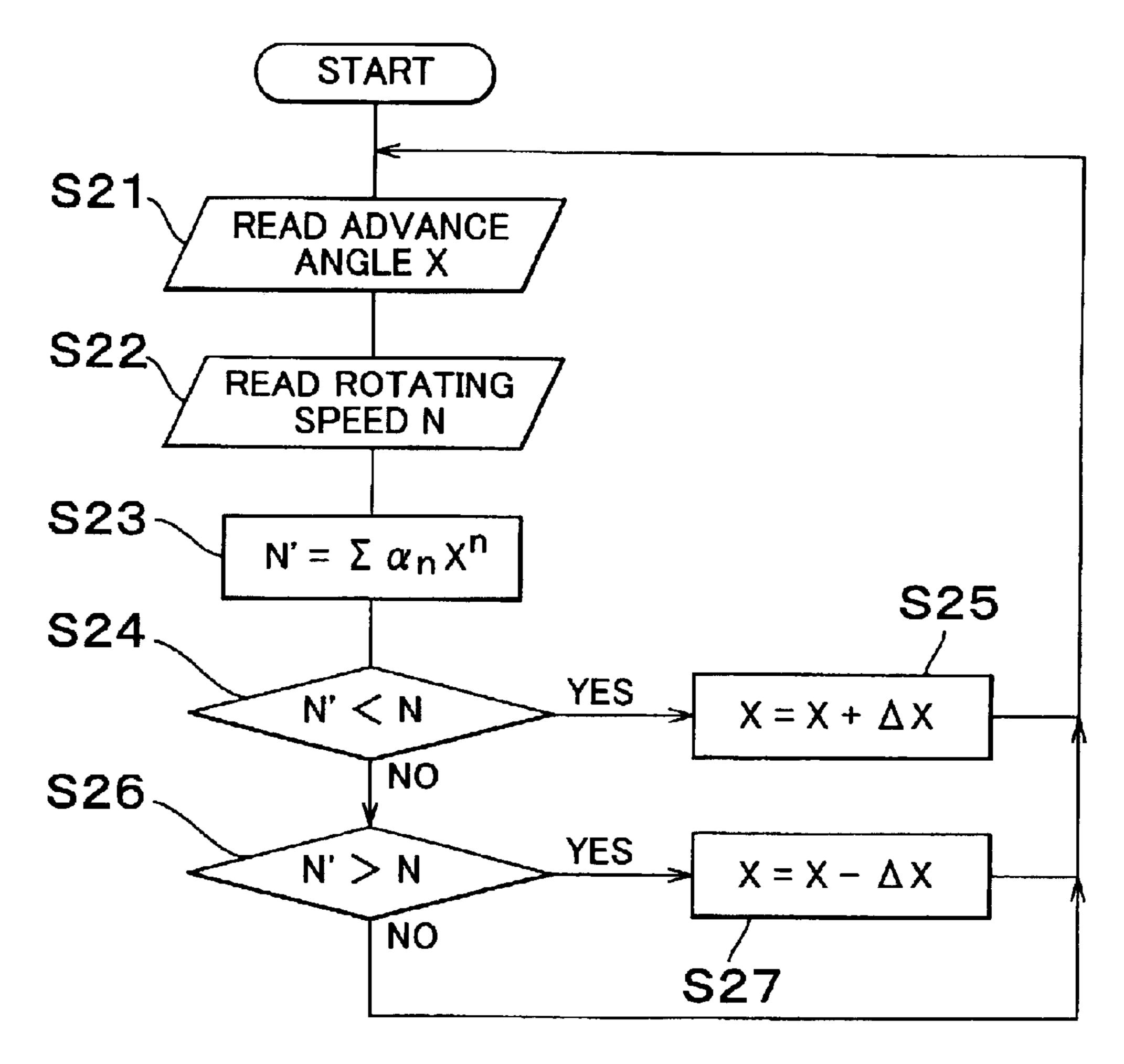
N': ESTIMATED VALUE OF MOTOR ROTATING SPEED OBTAINED BY STORED DATA MAP OR EQUATIONS
