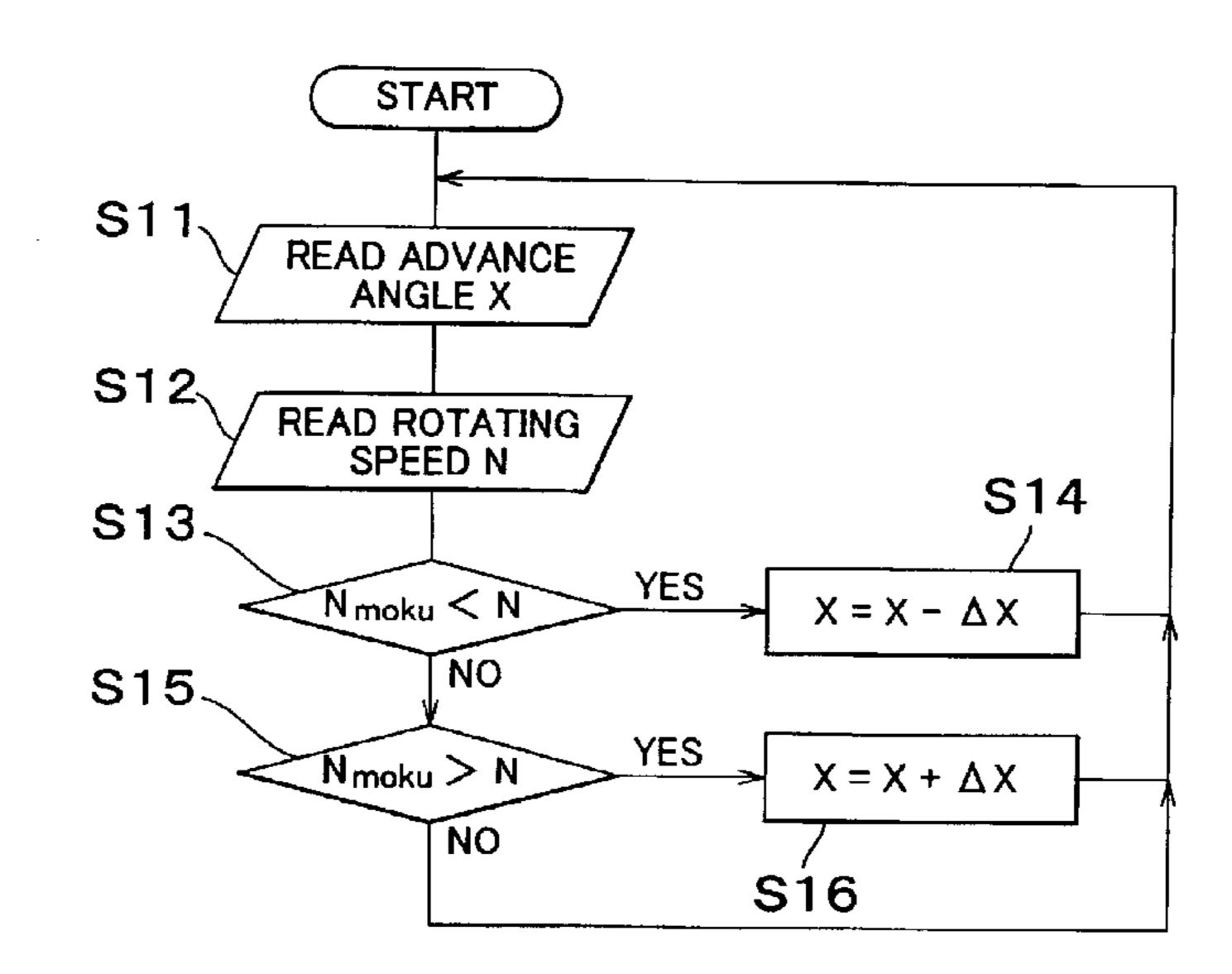
Nmoku: TARGET VALUE OF MOTOR ROTATING SPEED
