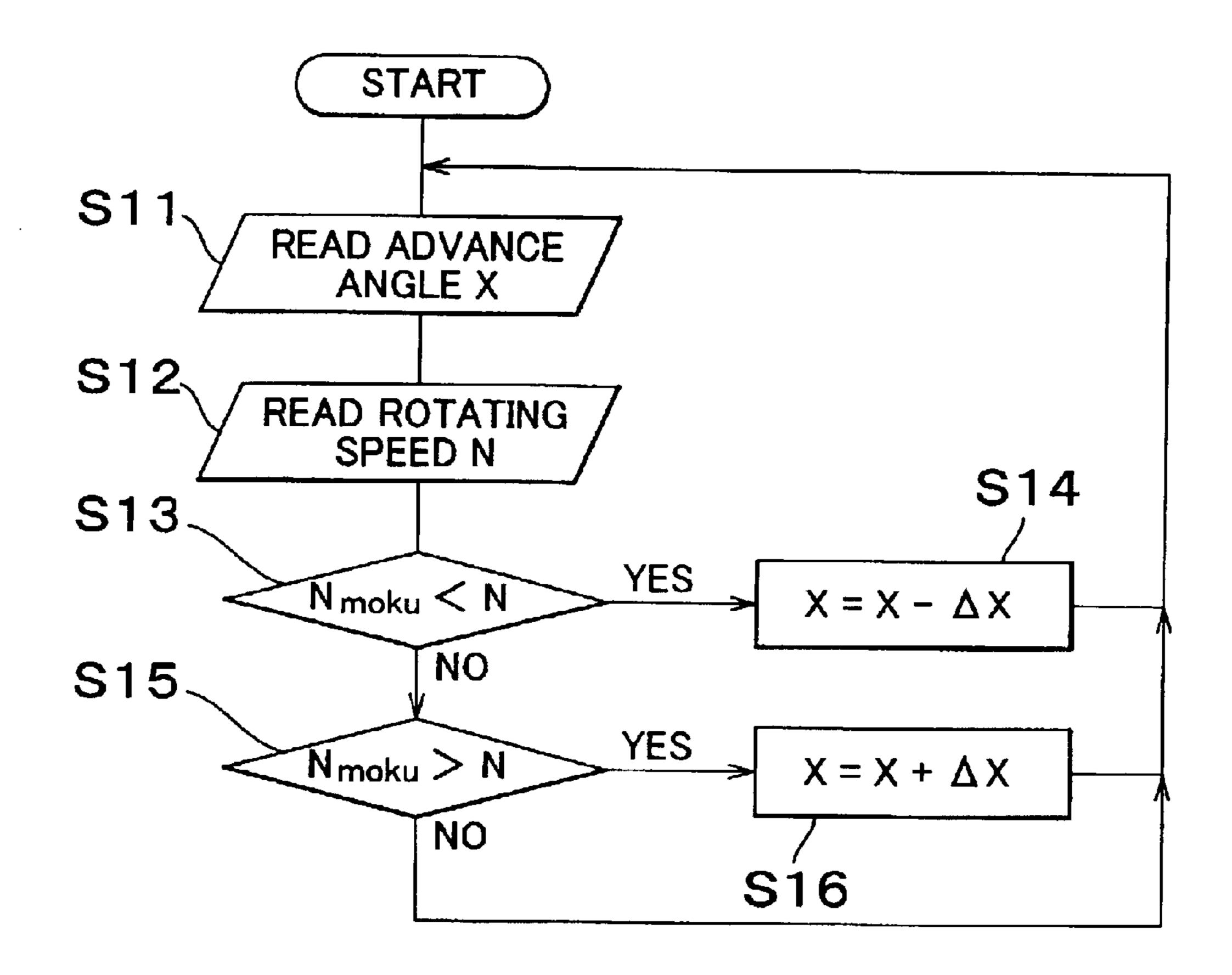
N<sub>moku</sub>: TARGET VALUE OF MOTOR ROTATING SPEED
