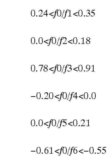
According to this embodiment, by sharing the greater part of the positive refractive power of the overall projection lens system by the third lens which is a glass lens element, the drift of the focus performance by temperature change is reduced.
