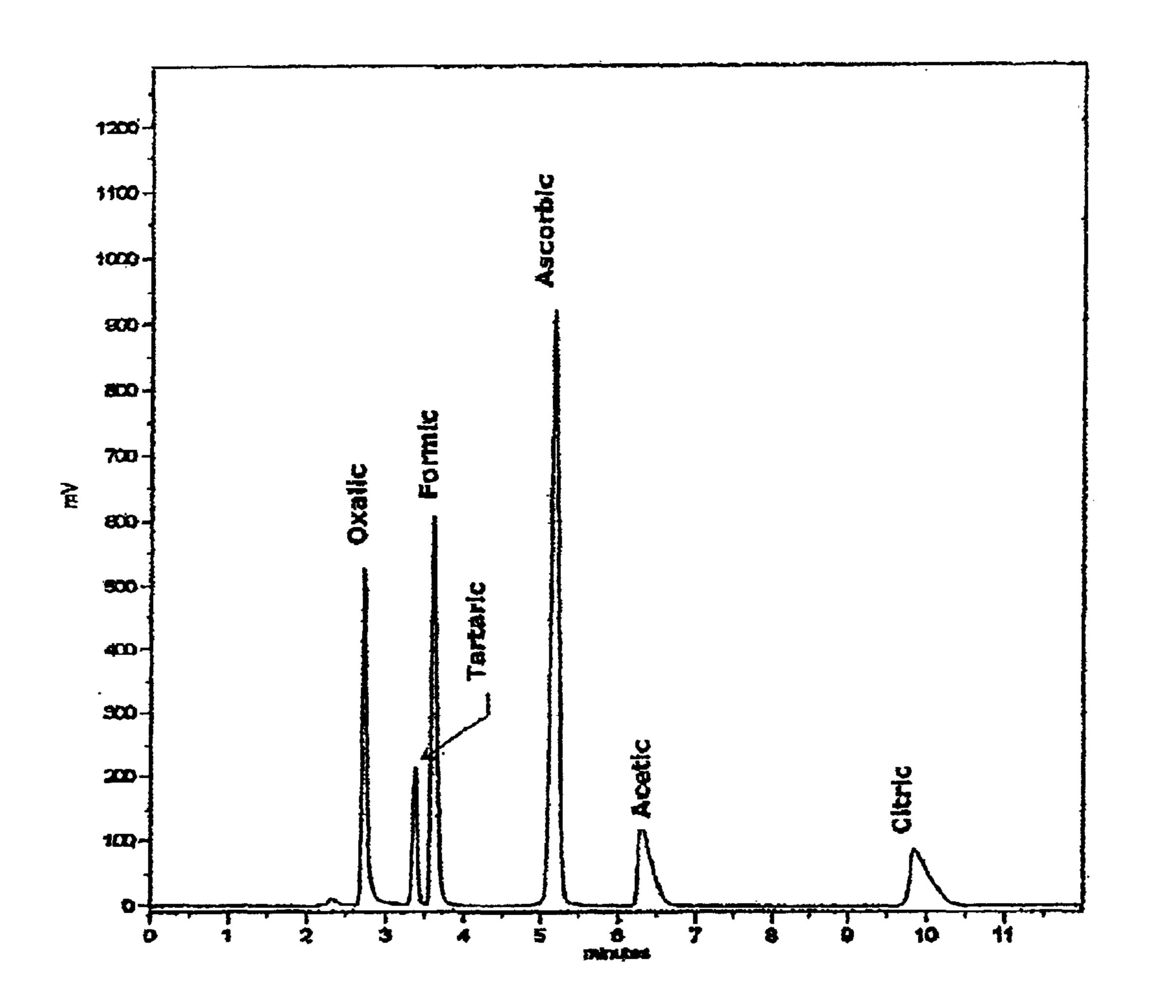
FIGURE 4. RETENTION TIME STABILITY OF CITRIC ACID ON DI-DODECYLMETHYLSILYLETHYL BONDED SILICA, 250 x 4.6 mm, 60A, 5u
