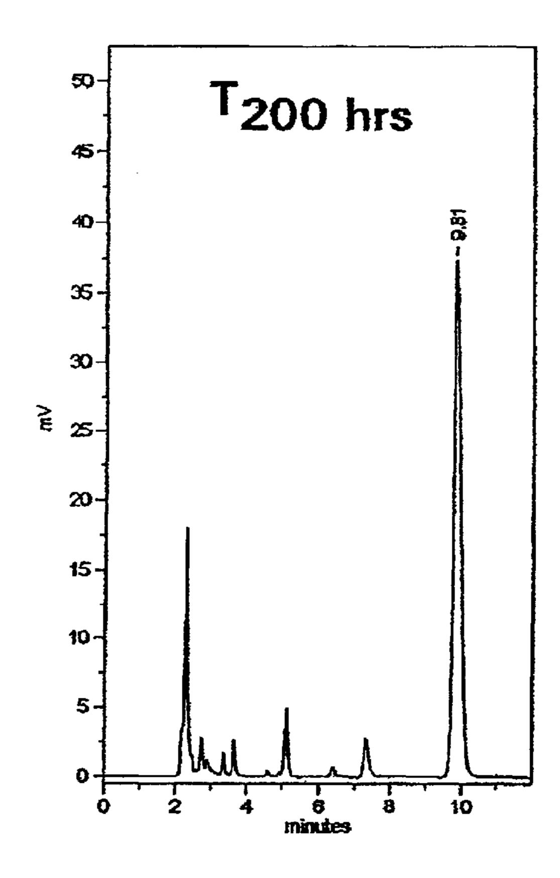
FIGURE 5. RETENTION TIME INSTABILITY OF CARBOXYLIC ACIDS ON CONVENTIONAL C18 BONDED SILICA, 250 x 4.6 mm, 60A, 5u
