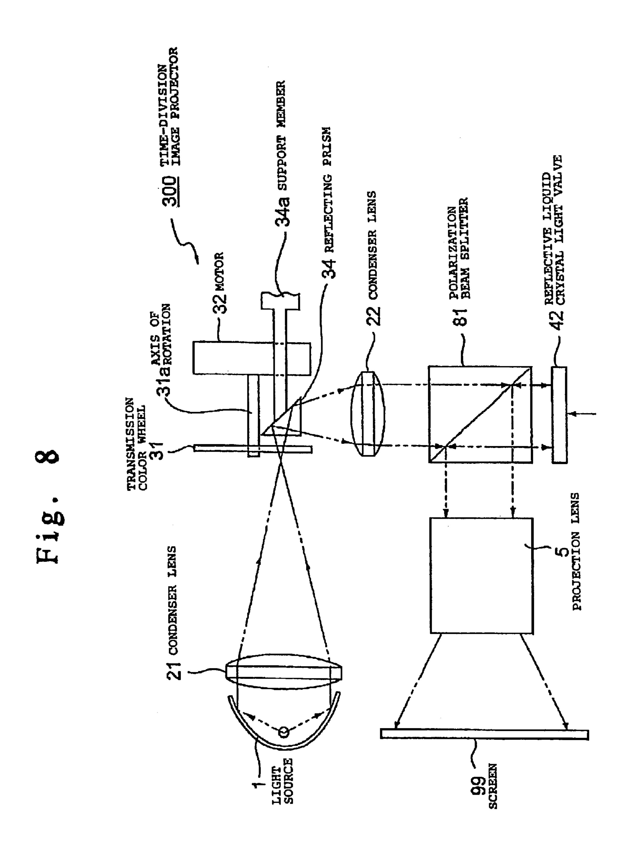
TIME-DIVISION IMAGE PROJECTOR MEMBER PRISM 22 CONDENSER LENS 5 PROJECTION AXIS OF ROTATION TRANSMISSION COLOR WHEEL 31
