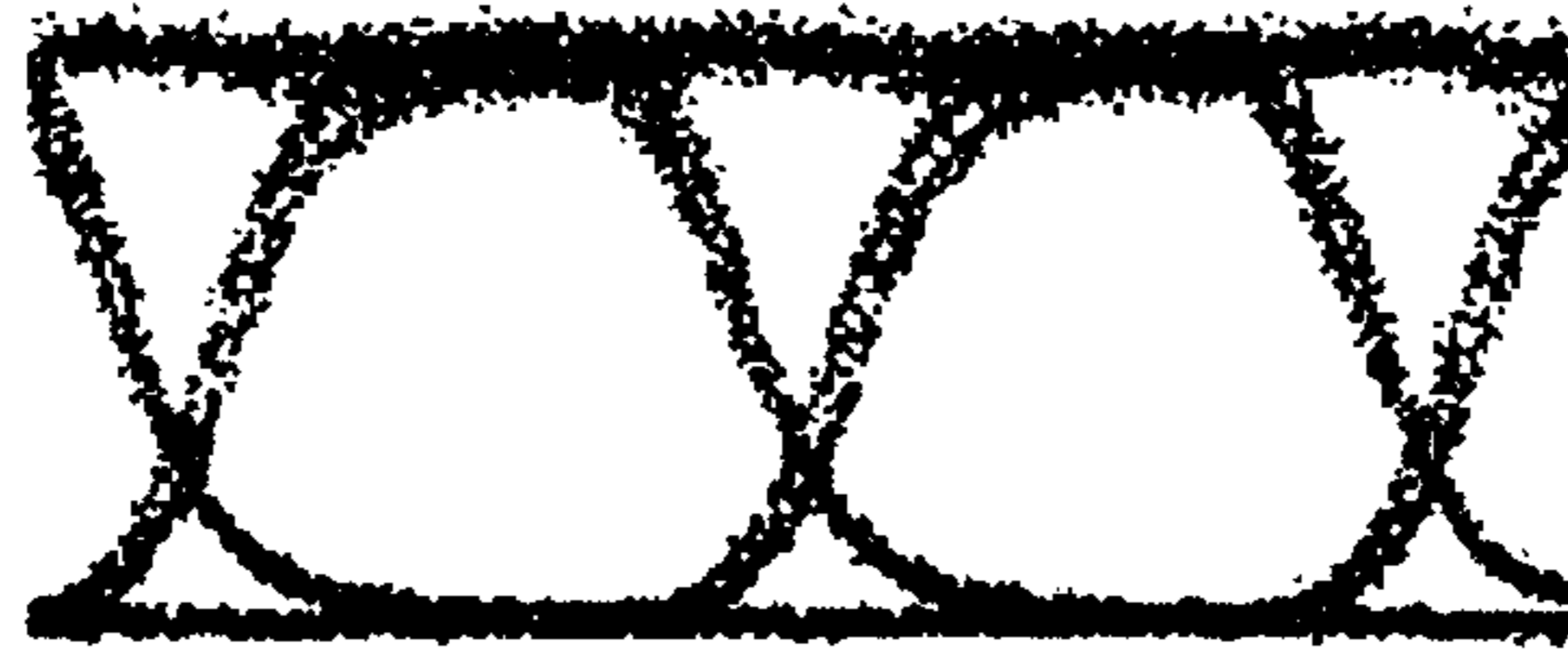
INPUT OPTICAL SIGNAL INTENSITY MODULATED IN 2.5 Gb/S (EXTINCTION RATIO : 15.52dB)
