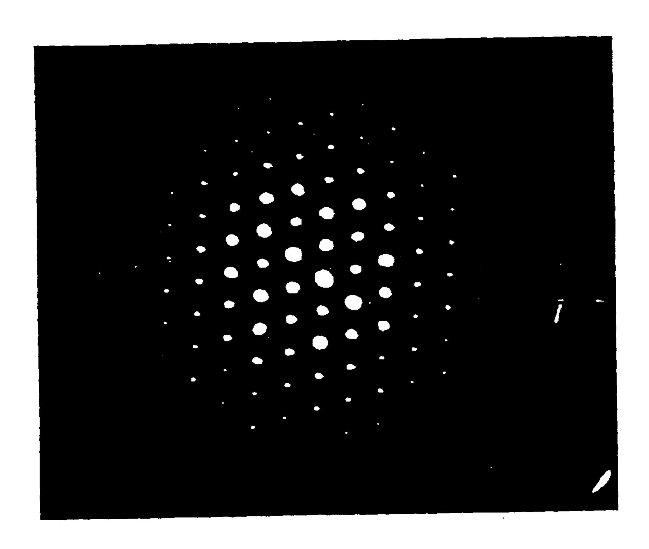
SELECTED-AREA ELECTRON DIFFRACTION OF SINGLE-CRYSTAL Mn-Zn FERRITE POWDER
