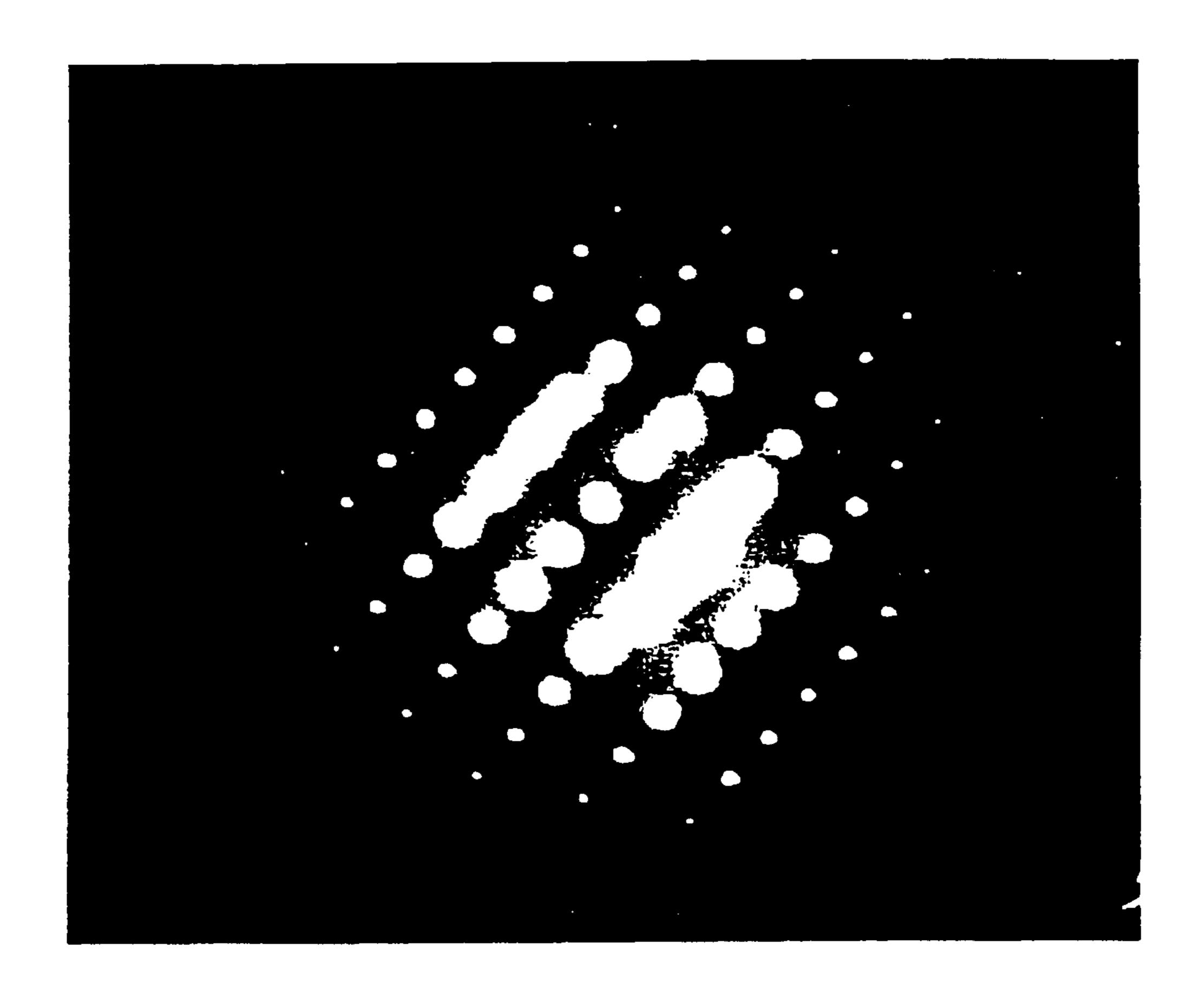
SELECTED-AREA ELECTRON DIFFRACTION OF SINGLE-CRYSTAL Ni-Zn FERRITE POWDER
