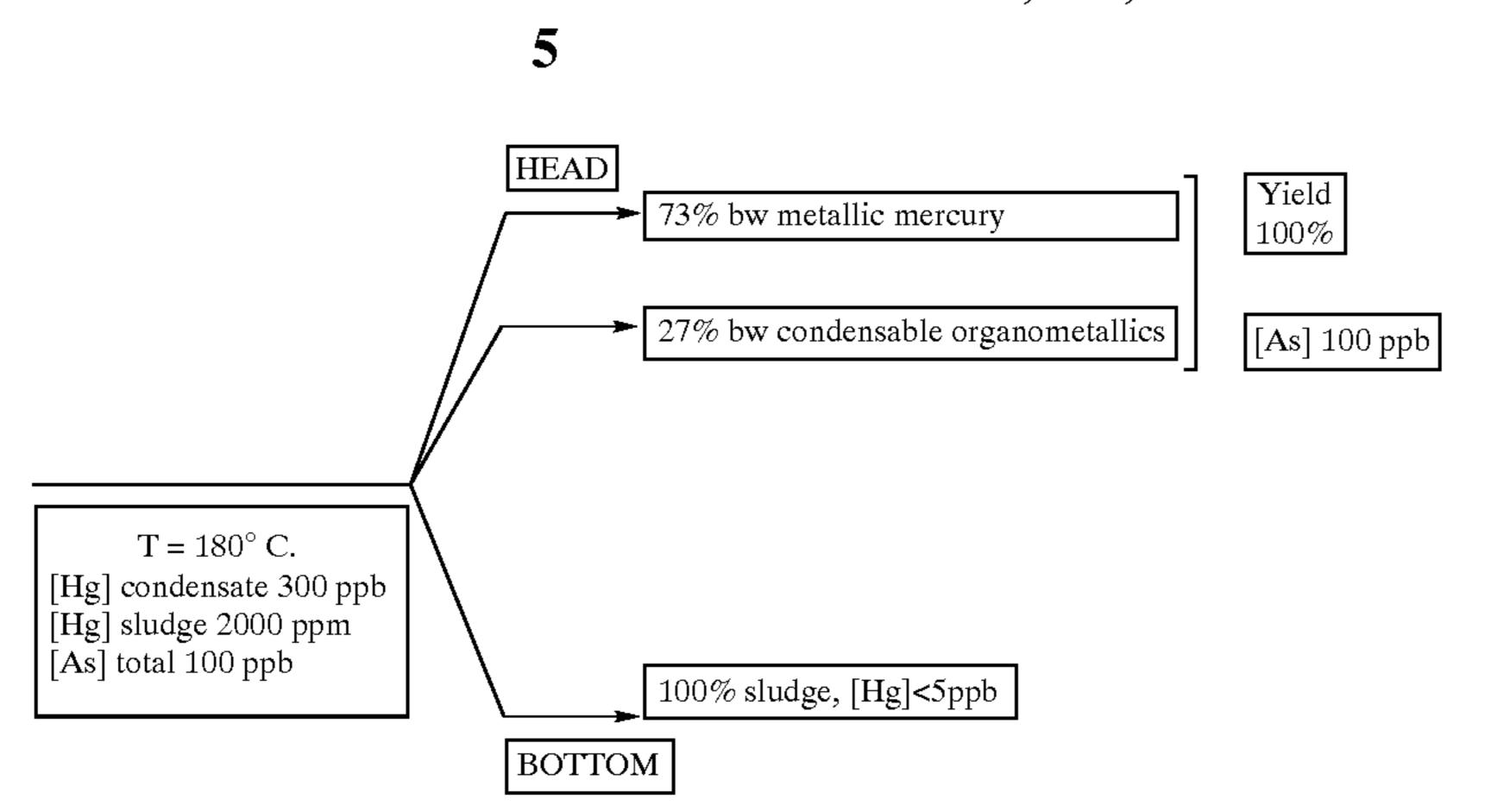
The pre-treated feed could then be sent to the units for steps b) and c).
