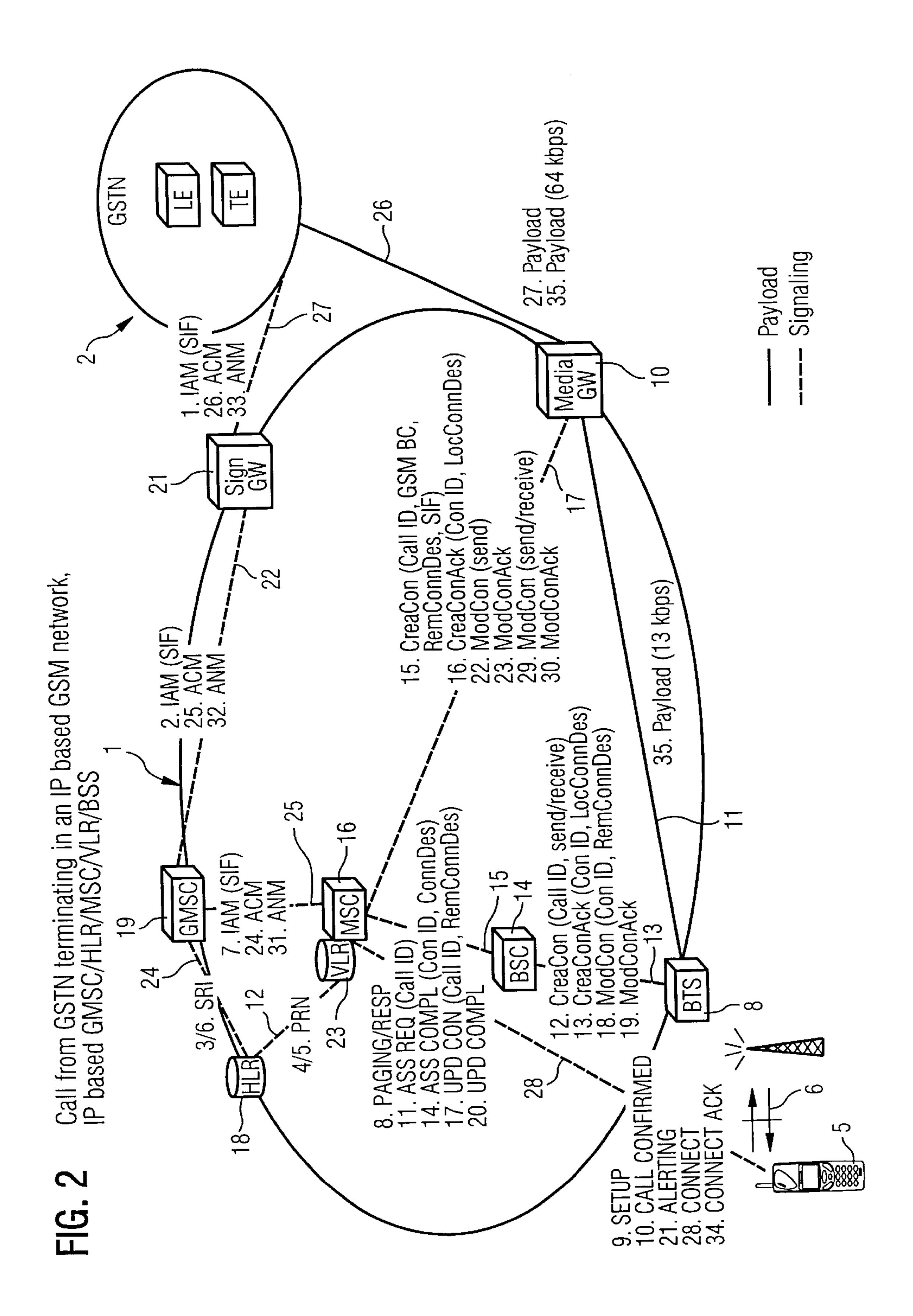
(64 kbps) (64kb) Signaling 127. 135. Payload Payload 31  $\sim$ Media GW 101. 133. 32 CreaCon (Call ID, GSM BC, RemConnDes, SIF2)
