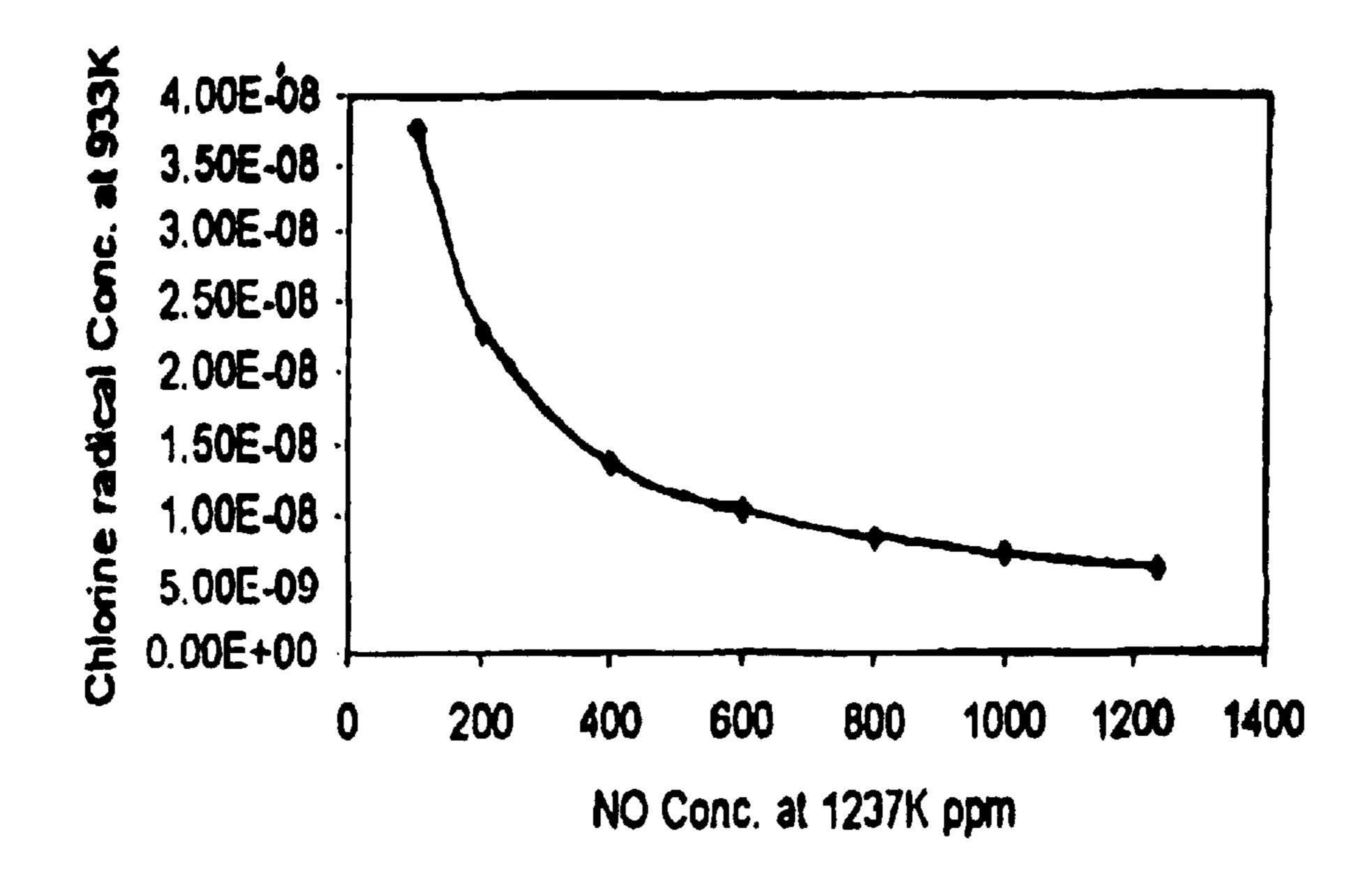
NO Conc. Effect on the Chlorine radical existence Flue gas composition: CO2: 0.1444, H2O: 0.0569,
