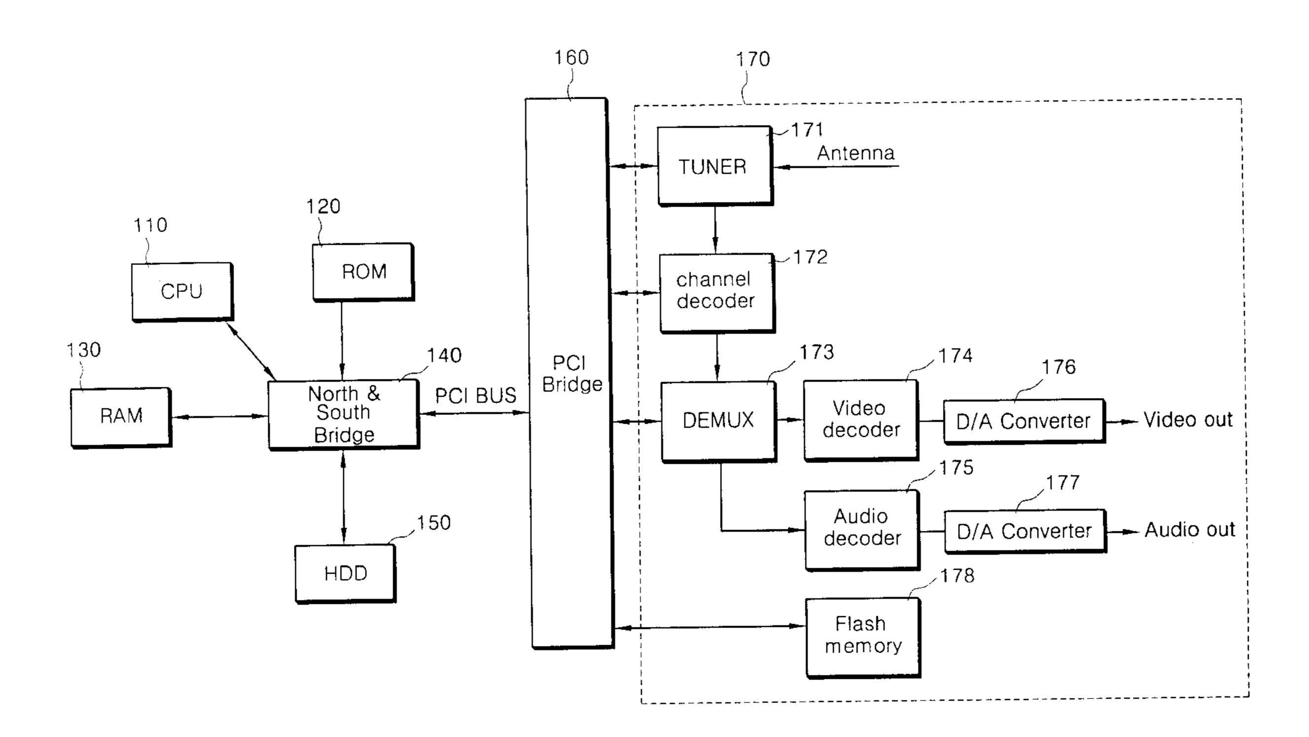
Video decoder Audio decoder channel decoder **DEMUX** TUNER PCI Bridge
